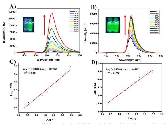
Fig. 3 Emission spectra of compounds (A) 7 (10  $\mu$ M,  $\lambda_{ex}$  = 350 nm) and (B) 8 (1  $\mu$ M,  $\lambda_{ex}$  = 350 nm), recorded in DMSO-glycerol mixtures with increasing glycerol content from 0% to 99%. Photographs captured under a UV 365 nm lamp are shown above each spectrum. Graphs illustrate the linear relationship between log I (fluorescence intensity) and log  $\eta$  (viscosity) of compounds **7** (C) and **8** (D).
