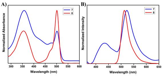
Fig. 1 (A) Normalized absorption (10  $\mu$ M) and (B) normalized emission spectra of compounds **7** and **8** in DCM (2  $\mu$ M,  $\lambda_{ex}$  = 350 nm).
