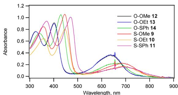
Fig. 5 UV-visible spectra of 19-substituted bilin-1-ones **12–14** and bilin-1-thiones **9–11**.  $2 \times 10^{-5}$  M in  $\text{CH}_2\text{Cl}_2$  at 298 K.
