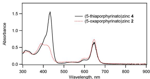
Fig. 3 UV-visible spectra of (5-thiaporphyrinato)zinc **4** and (5-oxaporphyrinato)zinc **2**,  $1.35 \times 10^{-5}$  M in  $\text{CHCl}_3$ .
