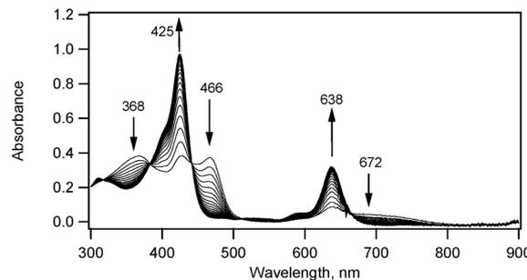
Fig. 6 UV-visible spectral changes of  $1 \times 10^{-5}$  M 19-phenylsulfanylbilin-1-thione **11** and 0.1 mM zinc acetate in 50% (v/v) acetonitrile in water at 298 K. Spectra were recorded every 4 seconds.
