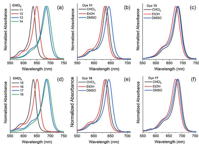
Fig. 2 Normalized UV-Vis absorption spectra for the solution of squaraines (a) **11–14** and (d) **15–18** in chloroform and squaraines (b) **11**, (c) **13**, (e) **15**, and (f) **17** in different organic solvents ( $\sim 10^{-6}$  mol L $^{-1}$ ).
