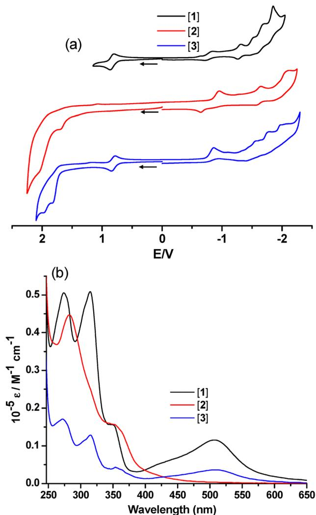
Fig. 5 (a) Cyclic voltammograms and (b) UV-Vis spectra of the complexes **1–3** recorded in  $\text{CH}_3\text{CN}$ . The voltammograms were recorded against the  $\text{Ag}/\text{AgCl}$  reference electrode and glassy carbon working electrode, and the potentials were adjusted against  $\text{Fc}/\text{Fc}^+$ .
