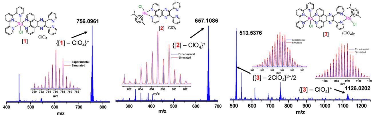
Fig. 2 Molecular structures of the complexes **1–3** and their corresponding HRMS spectra recorded in  $\text{CH}_3\text{OH}$ . The inset shows the isotopic distribution pattern of the molecular ion peaks.
