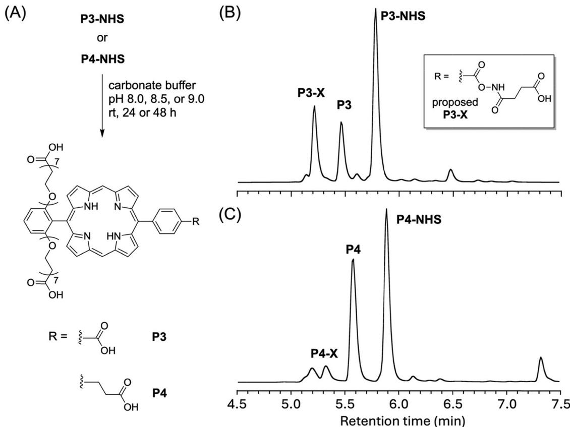
Fig. 1 (A) Hydrolysis of **P3-NHS** and **P4-NHS** in carbonate buffer/10% DMSO. Panels B and C: Reversed-phase C18 HPLC trace with absorption spectral detection of crude hydrolysis mixtures (50 mM, pH 9.0) after 2 h at room temperature for **P3-NHS** (B) or **P4-NHS** (C).
