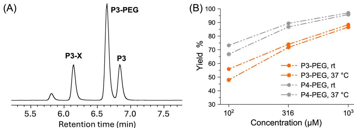
Fig. 8 (A) Reversed-phase C18 HPLC trace with absorption spectral detection of the crude conjugation mixtures of **P3-NHS** and mPEG<sub>4</sub>-NH<sub>2</sub> (entry 3, 100 µM, pH 9.0) in carbonate buffer/10% DMSO after 2 days. (B) Yield comparison among different porphyrin-NHS esters at different temperature and concentrations (log scale).
