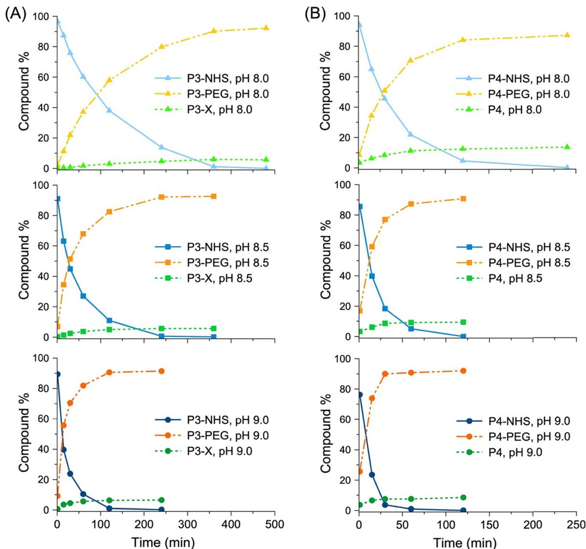
Fig. 6 Kinetics of conjugation of porphyrin-NHS esters with mPEG<sub>4</sub>-NH<sub>2</sub> in carbonate buffer/10% DMSO at various pH values at room temperature, assessed by HPLC-MS-Abs. (A) Data for **P3-NHS**; (B) data for **P4-NHS**.
