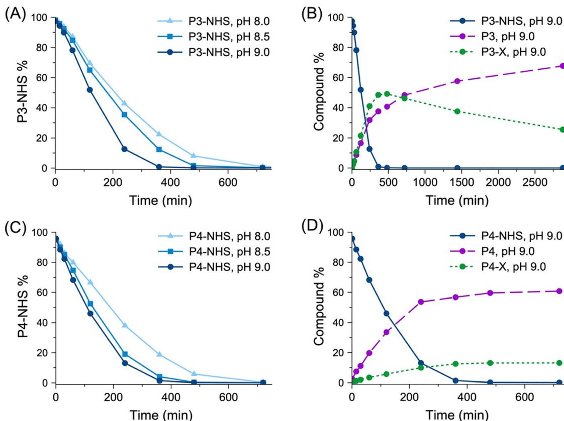
Fig. 2 Kinetics of hydrolysis of porphyrin-NHS esters in carbonate buffer/10% DMSO at given pH values at room temperature, assessed by HPLC-MS-Abs. (A) **P3-NHS** at three pH values over 12 h; (B) three major components of **P3-NHS** hydrolysis at pH 9.0 over 48 h; (C) **P4-NHS** at three pH values over 12 h; (D) three major components of **P4-NHS** hydrolysis at pH 9.0 over 12 h.
