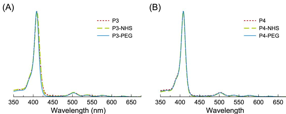
Fig. 5 Absorption spectra of porphyrins (normalized at the respective Soret bands) in DMSO at room temperature: (A) **P3** (dotted red trace), **P3-NHS** (dashed green trace), and **P3-PEG** (solid blue trace). (B) **P4** (dotted red trace), **P4-NHS** (dashed green trace), and **P4-PEG** (solid blue trace).
