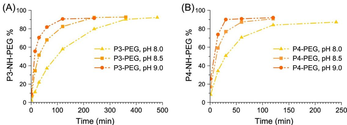
Fig. 7 Kinetics of conjugation reactions of porphyrin-NHS esters with mPEG<sub>4</sub>-NH<sub>2</sub> in carbonate buffer/10% DMSO at various pH values at room temperature, assessed by HPLC-MS-Abs. (A) Conjugations of **P3-NHS**; (B) conjugations of **P4-NHS**.
