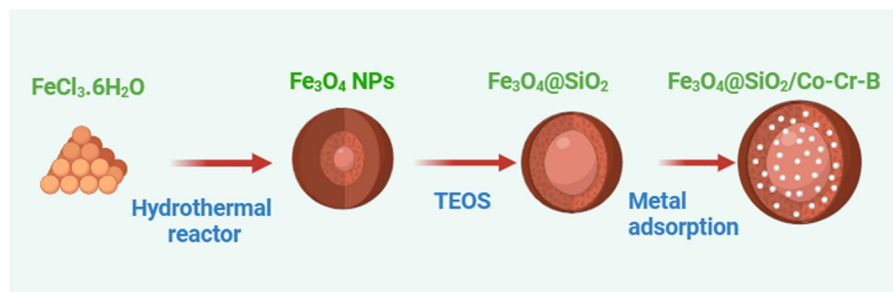
Fig. 1 Schematic representation of catalyst preparation.
