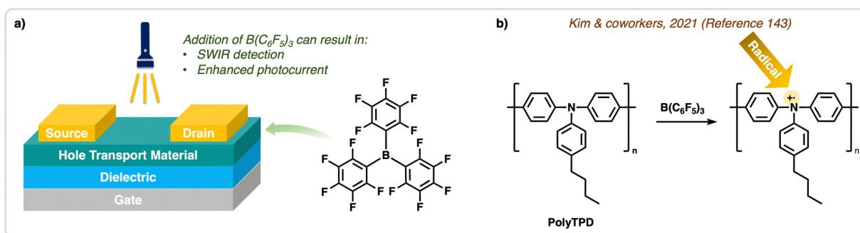
**Fig. 14** Application of  $B(C_6F_5)_3$  in OPTRs. (a) Structure of organic phototransistor devices used to detect various wavelengths of light. Addition of  $B(C_6F_5)_3$  in these types of devices can result in SWIR detection and enhanced photocurrent. (b) In the work done by Kim & coworkers,<sup>143</sup> doping of PolyTPD with  $B(C_6F_5)_3$  to generate radicals was done for applications in OPTRs.
