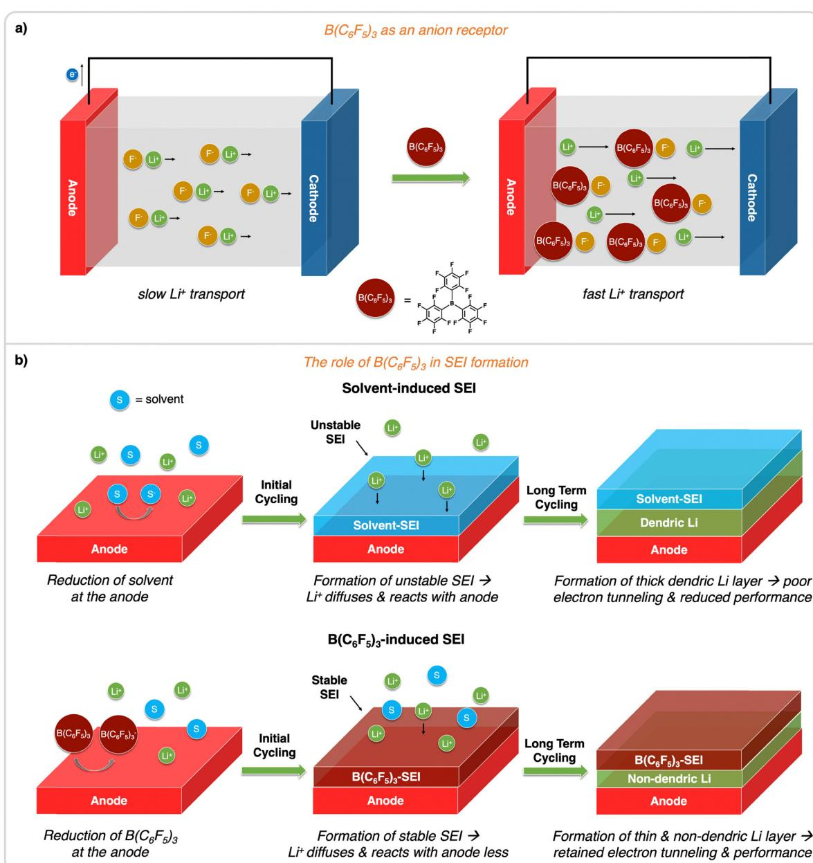
Fig. 8 The role of  $B(C_6F_5)_3$  in LIBs. (a)  $B(C_6F_5)_3$  as an anion receptor, which serves to aid in dissolution of LiF salts and increase the movement of Li<sup>+</sup>. (b)  $B(C_6F_5)_3$  as a sacrificial additive to LIBs to induce ideal SEI on the anode.
