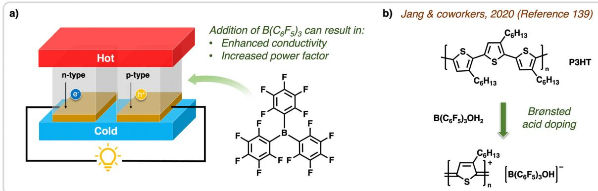
**Fig. 12** Application of  $B(C_6F_5)_3$  in OTEs. (a) Structure of an organic thermoelectric device used to convert heat into current. Using  $B(C_6F_5)_3$  to p-dope OTEs results in enhanced conductivity and increases the power factor of the devices. (b) In the work done by Jang & coworkers,<sup>139</sup> Brønsted acid doping was observed when mixing  $B(C_6F_5)_3$  (in the presence of water) with P3HT, which was used for OTEs and resulted in enhanced conductivity.
