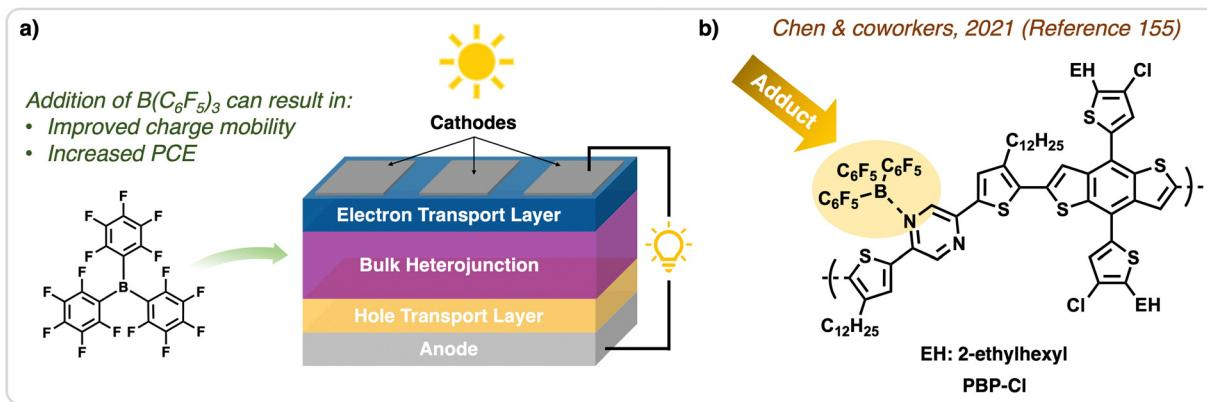
**Fig. 11** Application of  $B(C_6F_5)_3$  in OPVs. (a) Structure of an OPV used to harvest and convert solar radiation into current,  $B(C_6F_5)_3$  can be incorporated into the BHJ for increased charge mobilities and PCEs. (b) In the work done by Chen & coworkers,<sup>155</sup> adduct formation between the boron of  $B(C_6F_5)_3$  with the nitrogen on the pyrazine-based polymer, PBP-Cl, is observed, which was applied to OPVs for enhanced performance.
