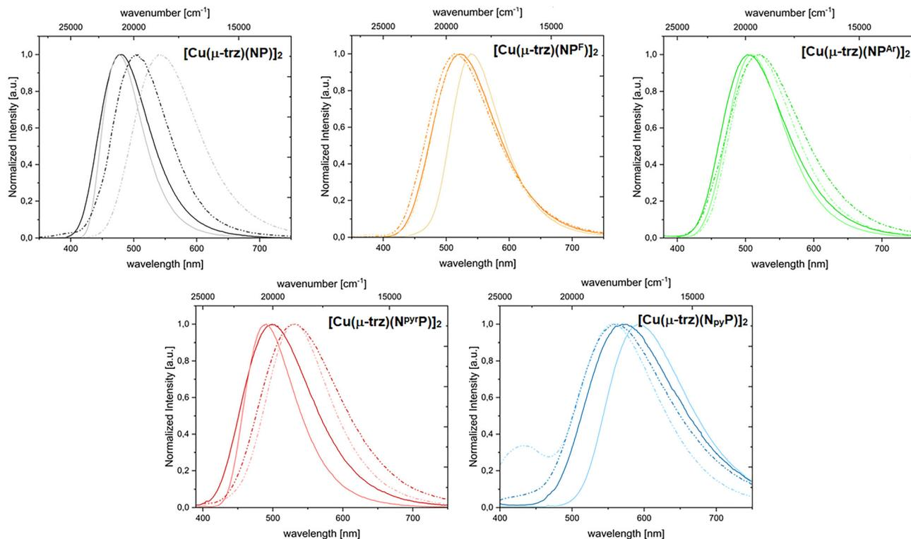
Fig. 4 Emission spectra of  $[\text{Cu}(\mu\text{-trz})(\text{NP})]_2$  (black),  $[\text{Cu}(\mu\text{-trz})(\text{NPF})]_2$  (orange),  $[\text{Cu}(\mu\text{-trz})(\text{NPAr})]_2$  (green),  $[\text{Cu}(\mu\text{-trz})(\text{NPyP})]_2$  (red) and  $[\text{Cu}(\mu\text{-trz})(\text{NpyP})]_2$  (blue) in the solid state (solid lines) and PMMA matrix (dashed lines). Vivid and faded colours refer to the data collected at 297 K and 77 K respectively.
