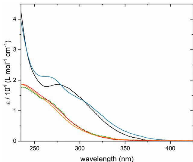
Fig. 3 UV-vis spectra collected in DCM at room temperature of  $[\text{Cu}(\mu\text{-trz})(\text{NP})]_2$  (black line),  $[\text{Cu}(\mu\text{-trz})(\text{NPF})]_2$  (orange line),  $[\text{Cu}(\mu\text{-trz})(\text{NPAr})]_2$  (green line),  $[\text{Cu}(\mu\text{-trz})(\text{NPyP})]_2$  (red line) and  $[\text{Cu}(\mu\text{-trz})(\text{NpyP})]_2$  (blue line).
