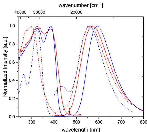
Fig. 5 Excitation and emission spectra of  $[\text{Cu}(\mu\text{-trz})(\text{N}_{\text{py}}\text{P})]_2$  in the solid state (solid lines) and in the PMMA matrix (dashed lines) at room temperature (red) and 77 K (blue).
