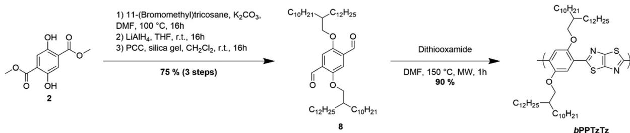
Scheme 4 Synthesis of polymer **bpPTzTz**.
