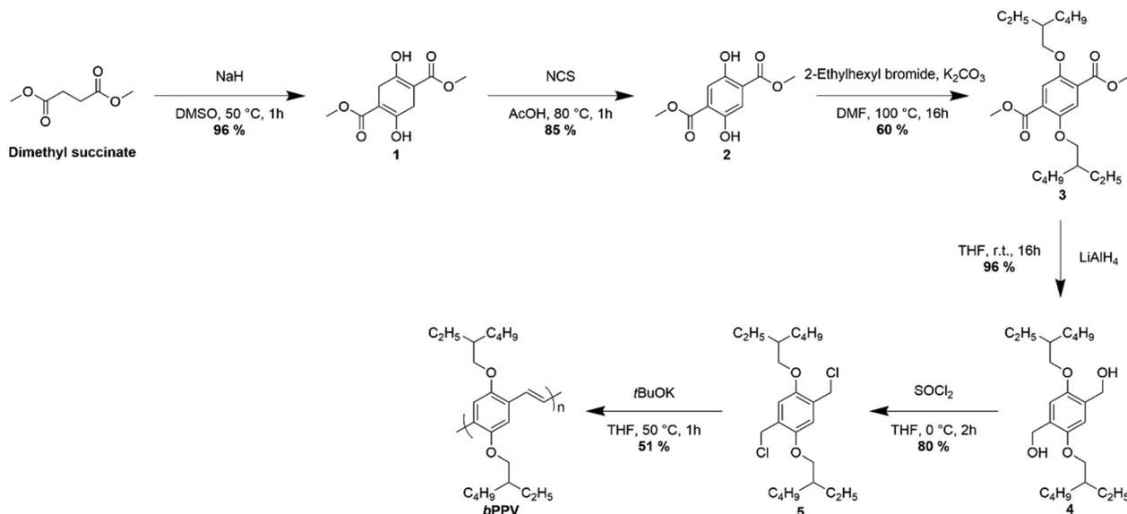
Scheme 2 Synthesis of polymer **bPPV**.
