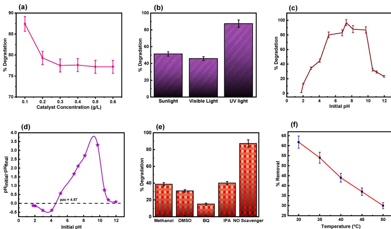
Fig. 5 Impact of (a) catalyst dose, (b) various lights, (c) pH, (d) pzc studies, (e) scavengers, and (f) temperature. Error bars represent the standard deviation from triplicate experiments with 95% confidence intervals.
