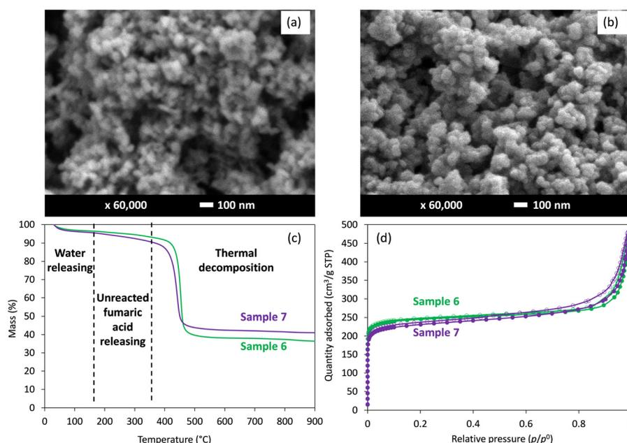
Fig. 4 (a) SEM images of sample 6 and (b) sample 7. (c) Thermograms under air of sample 6 (green curve) and sample 7 (purple curve). (d) Nitrogen adsorption–desorption isotherms at  $-196$  °C for sample 6 (green curve) and sample 7 (purple curve) (filled and open symbols represent adsorption and desorption isotherms, respectively).
