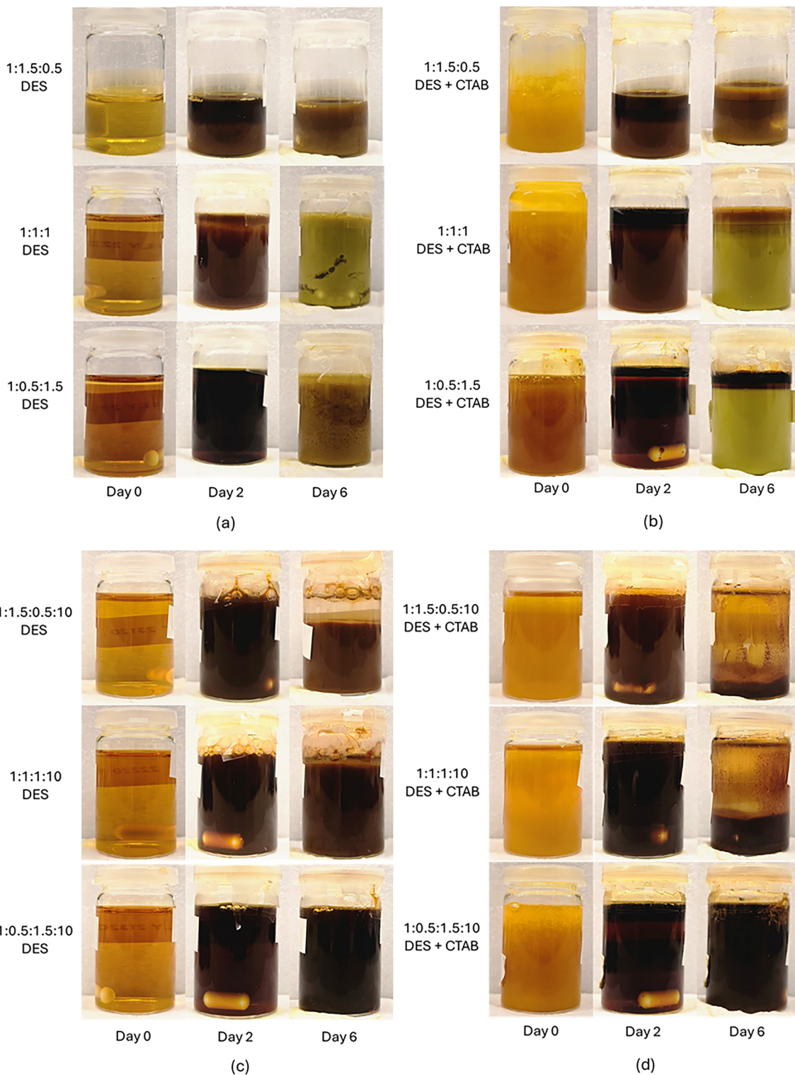
Fig. 1 Pictures of \text{Fe}(\text{NO}_3)_3 dissolved in unhydrated and hydrated DES kept at 70 °C. (a) \text{Fe}(\text{NO}_3)_3 in unhydrated DES w/o CTAB, (b) \text{Fe}(\text{NO}_3)_3 in unhydrated DES w/CTAB, (c) \text{Fe}(\text{NO}_3)_3 in hydrated DES w/o CTAB, and (d) \text{Fe}(\text{NO}_3)_3 in hydrated DES w/CTAB. The pictures are taken at day 0, day 2 and day 6 after dissolving the salt. The nanoparticles were separated by injecting this solution into DI water, after 7 days stored at 70 °C, after dissolving the salt.
