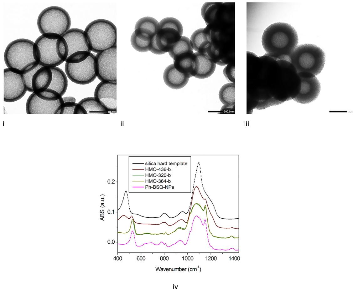
Fig. 4 TEM images (scale 200 nm) of (i) HMO-436-b, with an average diameter of  $436 \pm 18$  nm and a shell thickness of  $55 \pm 5$  nm, (ii) HMO-320-c, with an average diameter of  $320 \pm 13$  nm and a shell thickness of  $50 \pm 10$  nm, and (iii) HMO-364-c, with an average diameter of  $364 \pm 22$  nm and a shell thickness of  $87 \pm 6$  nm. (iv) Comparison of MIR spectra for HMO-365-b, HMO-320-b, and HMO-364-b and the reference spectra (silica hard template and Ph-BSQ-NPs).
