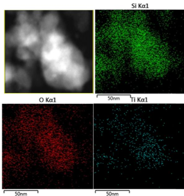
Fig. 6 EDX-SEM images of the Ti-UVM-7 material.
