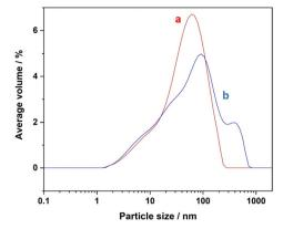
Fig. 7 Particle size distribution curves of (a) UVM-7 and (b) Ti-UVM-7 supports loaded with A26 suspended in water media.
