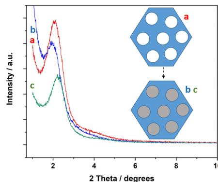
Fig. 4 Low-angle XRD patterns of (a) UVM-7, (b) UVM-7 loaded with Zenith A26 and (c) with neem oil.
