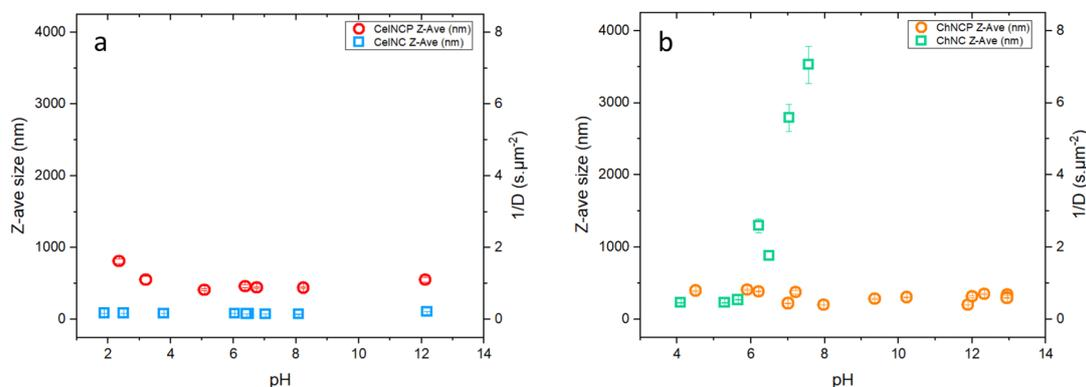
Fig. 3 Dimensions (equivalent sphere diameter) and inverse diffusion coefficient ( $1/D$ ) for polysaccharide cellulose and chitin nanocrystals dispersed in aqueous medium at different pH: (a) pristine and phosphorylated cellulose nanocrystals (CellNC, CellNC-P); (b) pristine and phosphorylated chitin nanocrystals (ChitNC, ChitNC-P). For most samples, the error bars displayed in the figure are smaller than the symbols size.
