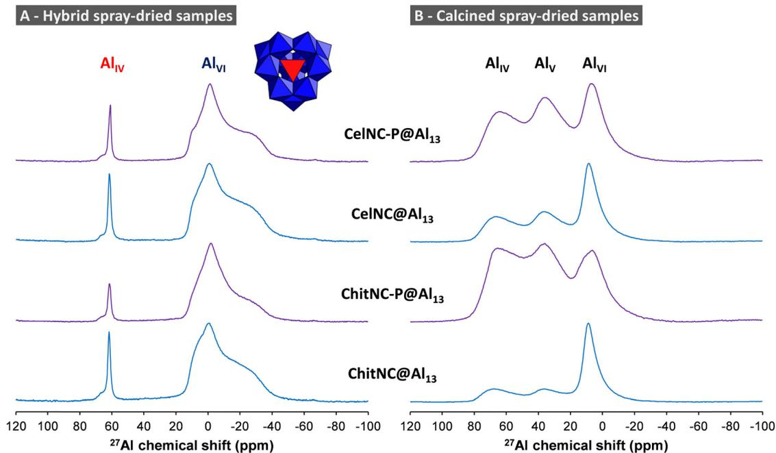
Fig. 13  $^{27}\text{Al}$  single pulse spectra recorded at  $\nu_0(^{27}\text{Al}) \equiv 156.3$  MHz and  $\nu_{\text{MAS}} = 15$  to 20 kHz. The scheme of the  $\text{Al}_{13}$  cluster highlights the central  $\text{AlO}_4$  tetrahedra (in red) surrounded by the 12  $\text{AlO}_6$  octahedra (in blue).
