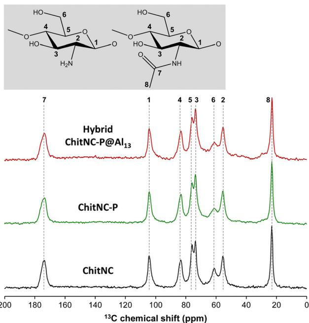
**Fig. 11** <sup>13</sup>C(<sup>1</sup>H) CP-MAS spectra of spray-dried microparticles obtained from different polysaccharide colloids: pristine chitin nanocrystals (ChitNC), phosphorylated ChitNC (ChitNC-P), and ChitNC-P in interaction with Al<sub>13</sub> (ChitNC-P@Al<sub>13</sub>). The spectra were recorded at  $\nu_0(^{13}\text{C}) \equiv 75.4$  MHz and  $\nu_{\text{MAS}} = 12$  kHz (see Experimental), acquiring 4096 scans.
