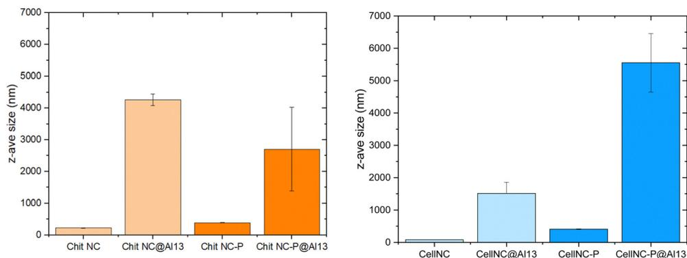
**Fig. 6** Z-averaged hydrodynamic diameter measured by DLS for hybrid suspensions of (a) chitin and (b) cellulose nanocrystals after phosphorylation or not, in the presence or absence of Al<sub>13</sub> clusters.
