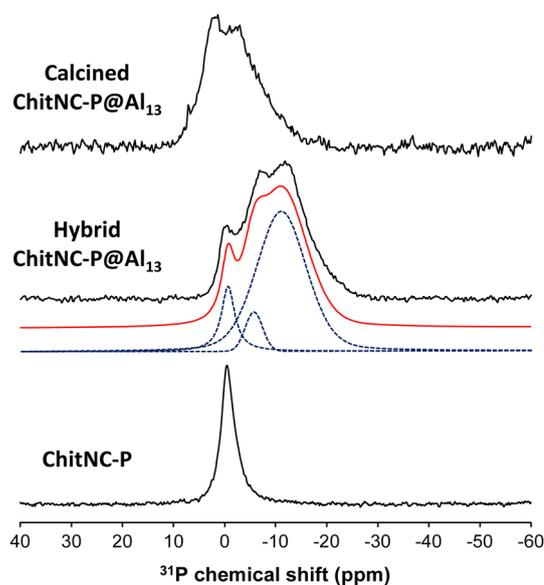
**Fig. 12** <sup>31</sup>P(<sup>1</sup>H) CP-MAS spectra recorded at  $\nu_0(^{31}\text{P}) \equiv 242.8$  MHz and  $\nu_{\text{MAS}} = 12$  kHz ( $\tau_c = 2$  ms), acquiring 64 scans for the ChitNC-P precursor, and 256 for the hybrid and calcined materials. The spectrum of the hybrid (middle) was fitted using the peak's characteristics of the ChitNC-P precursor and two other peak functions freely optimized.
