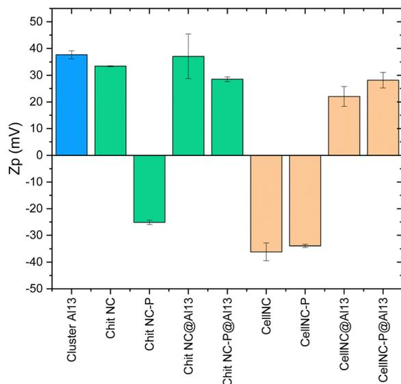
Fig. 7 Zeta potential measurements of hybrid suspensions at pH 4.5 for Al<sub>13</sub> clusters alone, polysaccharide nanocrystals phosphorylated (ChitNC-P, CellNC-P) or not (ChitNC, CellNC) alone, and in the presence of Al<sub>13</sub> (ChitNC@Al<sub>13</sub>, ChitNC-P@Al<sub>13</sub>, CellNC@Al<sub>13</sub>, CellNC-P@Al<sub>13</sub>).
