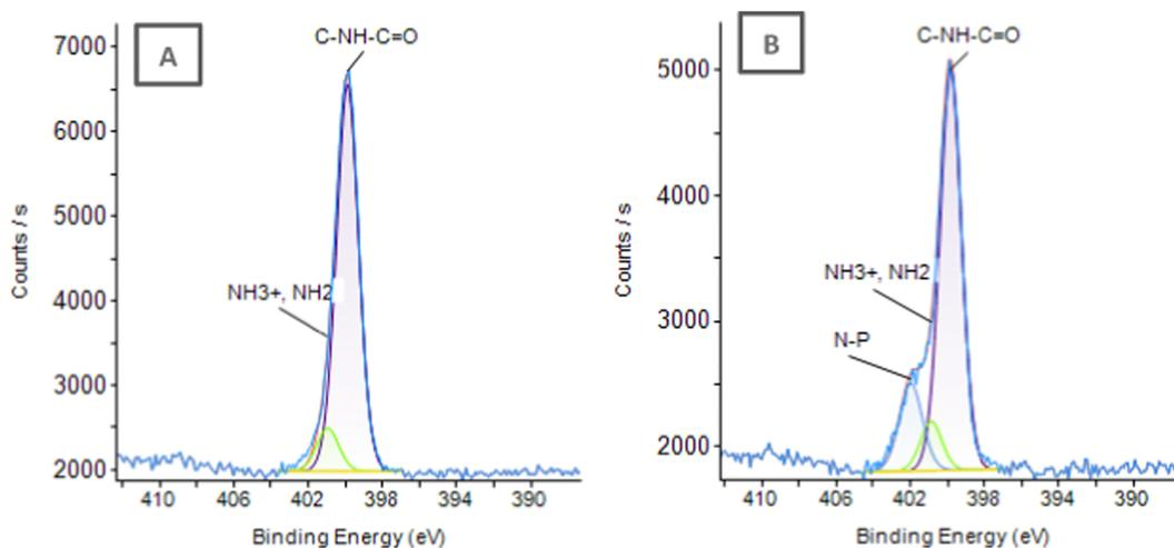
Fig. 1 N1s XPS spectra deconvolution for chitin nanocrystals before (A) (ChitNC) and after (B) (ChitNCP) reaction with POCl<sub>3</sub>.
