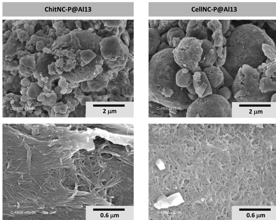
Fig. 8 SEM images of hybrid spray-dried microparticles obtained with phosphorylated polysaccharide NPs and  $Al_{13}$  clusters.
