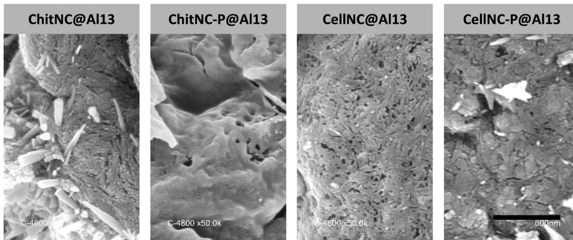
**Fig. 10** Surfaces of calcined spray-microparticles analyzed by SEM. The observed porosity is formed by the imprints of the polysaccharide NPs (removed during calcination in air). The crystalline shapes observed in some of the micrographs correspond to residual NaCl crystals formed by the presence of chlorine and sodium ions in the NCs and  $\text{Al}_{13}$  suspensions respectively.<sup>51</sup> The magnification is the same for all samples, and the scale bar represents 600 nm.
