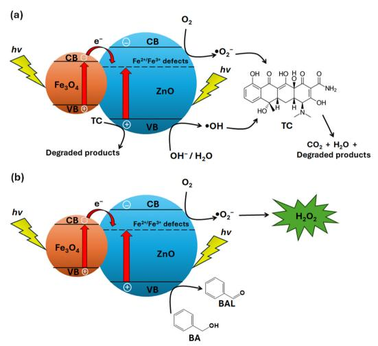
Fig. 7 Illustration of the photocatalytic mechanisms in Fe<sub>3</sub>O<sub>4</sub>/ZnO heterostructures for (a) TC degradation and (b) H<sub>2</sub>O<sub>2</sub> production, under light irradiation.
