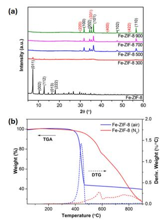
Fig. 3 (a) XRD patterns of uncalcined and calcined Fe-ZIF-8 at different temperatures (300, 500, 700, and 900 °C); (b) TGA and DTG of Fe-ZIF-8 under air and N2 atmosphere
