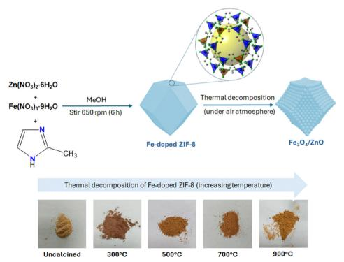
Fig. 1 Schematic representation of the synthesis of Fe-ZIF-8, followed by thermal decomposition under an air atmosphere to produce Fe<sub>3</sub>O<sub>4</sub>/ZnO heterostructures
