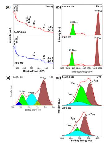
Fig. 5 XPS spectra of ZIF-8 500 and Fe-ZIF-8 500: (a) survey spectrum, (b) Zn 2p, (c) Fe 2p, and (d) O 1s.
