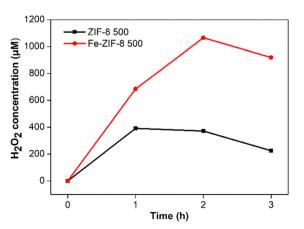
Fig. 8 Photocatalytic performance of ZIF-8 500 and Fe-ZIF-8 500 for H<sub>2</sub>O<sub>2</sub> production.
