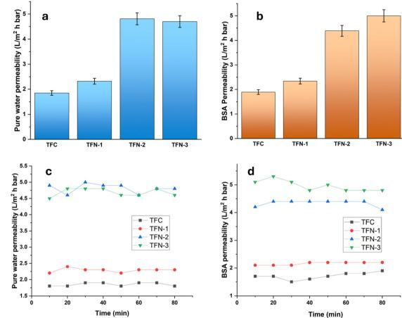
Fig. 4 Overall permeability of (a) water (b) BSA and time dependent permeability of (c) water and (d) BSA of the fabricated membranes.
