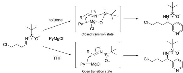
**Fig. 2** Choice of solvent to promote an open or closed transition state for Grignard addition to sulfinimine. Restricted rotation around the N–S bond, caused by dipole opposition, means rear approach from the in-coming nucleophile is blocked by the *tert*-butyl group in the open transition state.
