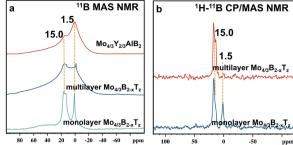
Fig. 3 (a)  $^{11}$ B MAS NMR spectra of Mo<sub>4/3</sub>Y<sub>2/3</sub>AlB<sub>2</sub>, multilayer Mo<sub>4/3</sub>B<sub>2-x</sub>T<sub>z</sub>, and monolayer  $Mo_{4/3}B_{2-x}T_z$ . (b)  $^1H-^{11}B$  CP/MAS NMR spectra of multilayer  $Mo_{4/3}B_{2-x}T_z$  and monolayer  $Mo_{4/3}B_{2-x}T_z$ .
