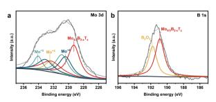
Fig. 2 High-resolution XPS spectra of monolayer  $Mo_{4/3}B_{2-x}T_z$ : (a) the Mo 3d region and (b) the B 1s region, and their fittings representing various species.
