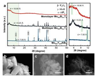
Fig. 1 (a) XRD patterns of 3D  $(Mo_{2/3}Y_{1/3})_2AlB_2$  and its 2D derivative  $Mo_{4/3}B_{2-x}T_z$  (monolayer and multilayer boridene); (b) SEM picture of 3D  $(Mo_{2/3}Y_{1/3})_2AlB_2$ ; (c) SEM picture of multilayer  $Mo_{4/3}B_{2-x}T_z$  boridene; and (d) SEM picture of monolayer Mo<sub>4/3</sub>B<sub>2-x</sub>T<sub>z</sub> boridene.
