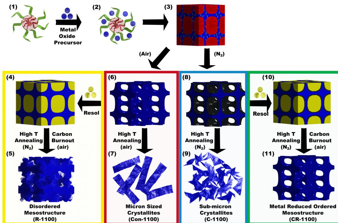
**Scheme 1** (1) Polymer micelles are used as templates for (2) metal oxide precursors (blue circles) where evaporative self-assembly leads to (3) a uniform architecture of micelles within an amorphous metal oxide network. (4)–(11) A range of processes were examined for structure preservation during high temperature treatments.
