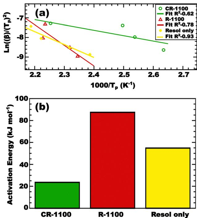
Fig. 6 (a) Kissinger plots derived from peak temperature ( $T_p$ ) of variable heat rate ( $\beta$ ) DSC endotherms of CR-1100 (green circles), R-1100 (red triangles), and resol only (yellow stars). (b) The linear best fits were used to determine the activation energies for resol polymerization in different local environments.
