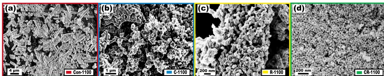
Fig. 2 SEM of samples annealed at 1100 °C (a) with conventional oxidizing conditions (Con-1100), or under nitrogen (b) with *in situ* carbon from the CASH method (C-1100), (c) with resol backfilling (R-1100), or (d) both CASH and resol back filling (CR-1100).
