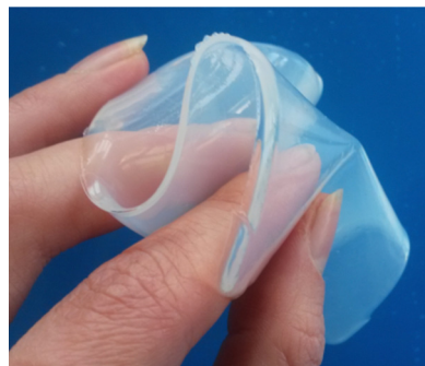
Fig. 11 Demonstrative flexibility of cellulose hydrogel.
