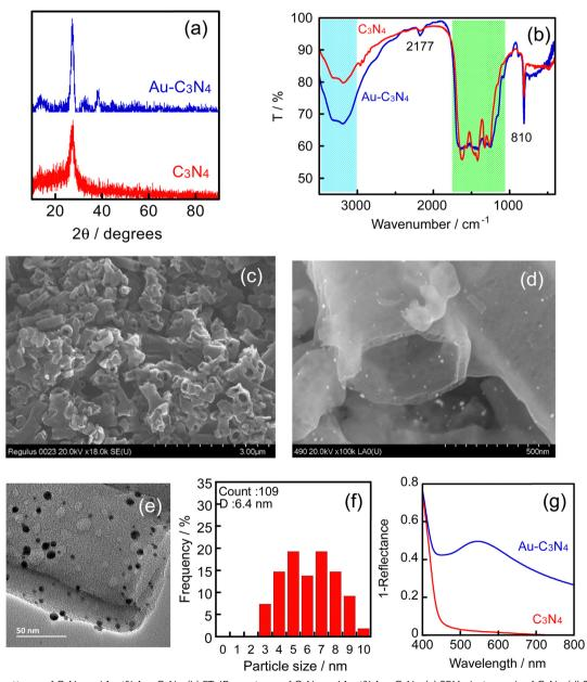
Fig. 1 (a) XRD patterns of  $C_3N_4$  and 1 wt%  $Au - C_3N_4$ , (b) FT-IR spectrum of  $C_3N_4$  and 1 wt%  $Au - C_3N_4$ , (c) SEM photograph of  $C_3N_4$ , (d) SEM photograph of 1 wt%  $Au-C_3N_4$ , (e) TEM photograph of 1 wt%  $Au-C_3N_4$ , (f) size distribution of Au nanoparticles loaded on  $C_3N_4$ , and (g) photoabsorption spectra of  $C_3N_4$  and 1 wt%  $Au-C_3N_4$
