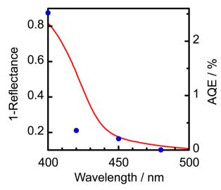
Fig. 4 An action spectrum of PBA production over Au-C<sub>3</sub>N<sub>4</sub>.
