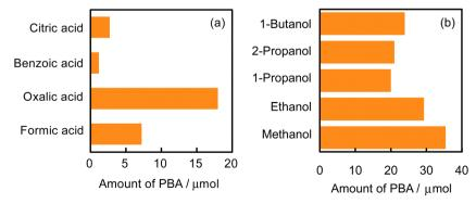
Fig. 5 Effects of (a) organic acid (100 μmol) in 2-propanol and (b) alcohol solvents containing OA (100 μmol) on production of PBA from AN and BAD via BAN in the suspension of 1 wt%  $Au-C_3N_4$  in the dark for 0.5 h and under subsequent light irradiation for 2 h.
