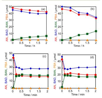
Fig. 2 Production of BAN ( $\blacksquare$ ) by condensation of AN ( $\bullet$ ) and BAD ( $\blacklozenge$ ) in 2-propanol suspensions under various conditions: (a) with no additive, (b) in the presence of 1 wt%  $Au-C_3N_4$  (50 mg), (c) in the presence of OA (100  $\mu$ mol), and (d) in the presence of OA (100  $\mu$ mol) and 1 wt% Au-C<sub>3</sub>N<sub>4</sub> (50 mg). PBA (▲) was not produced in all cases.
