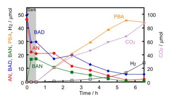
Fig. 3 Time courses of the amounts of BAD (♠), AN (♠), BAN (■), PBA ( $\triangle$ ), CO<sub>2</sub> ( $\nabla$ ) and H<sub>2</sub> ( $\square$ ) in a 2-propanol suspension of Au-C<sub>3</sub>N<sub>4</sub> in the presence of OA as an acid catalyst and a hole scavenger. The reaction was carried out in the dark for the first 0.5 h and under irradiation of UV light from a mercury lamp from 0.5 to 6.5 h.
