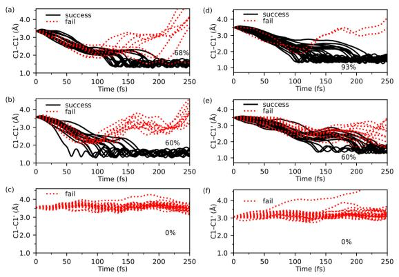
Fig. 4 Changes in C1-C1' distances during the NAMD trajectories of switches (a) T-I, (b) P-II, (c) 8, (d) 10, (e) 11 and (f) 17 compiled from our previous studies. 39.49 Percentage values refer to the proportion of trajectories that complete photocyclization within 250 fs
