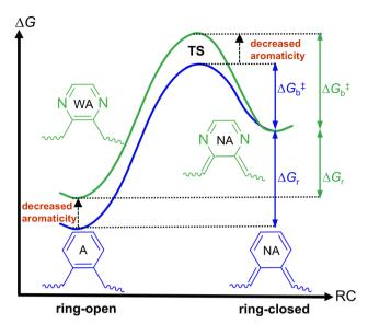
Fig. 1 Schematic illustration of how decreased aromaticity of the pyrazine  $\pi$ -linker (relative to the benzene  $\pi$ -linker) destabilizes the ring-open and TS forms, leading to a smaller  $\Delta G_r$  and a larger  $\Delta G_b^{\ddagger}$ . A, WA, and NA denote aromatic, weakly aromatic, and non-aromatic, respectively. Blue and green colors correspond to switches featuring benzene and pyrazine  $\pi$ -linkers, respectively. RC represents the reaction coordinate.
