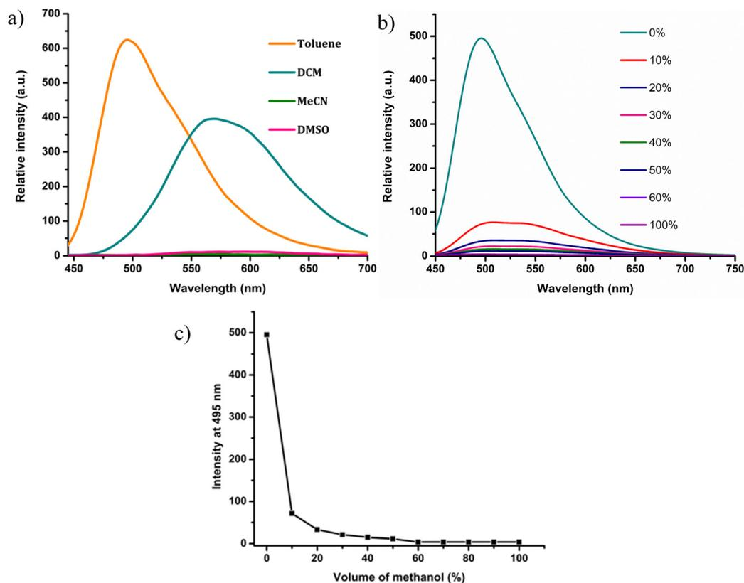
Fig. 4 Fluorescence spectra of 33  $\mu\text{M}$  solution of **3** (a) in different solvents, (b) in toluene in the presence of varying percentages of methanol, and (c) plot of percentage of methanol vs. emission intensity at 495 nm.
