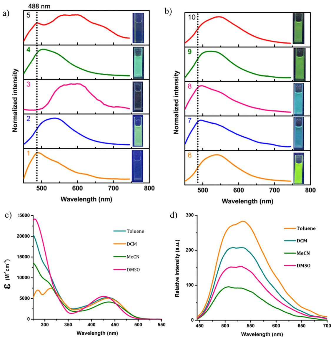
Fig. 2 (a) and (b) Emission spectra of the 33  $\mu\text{M}$  solution of compounds **1–10** in DMSO and their photographs under 365 nm UV lamp; (c) absorption and (d) emission spectra of 33  $\mu\text{M}$  solution of **9** in different solvents.
