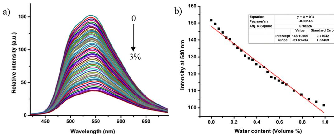
Fig. 5 (a) Fluorescence spectra of 33 μM solution of **3** in 1,4-dioxane with increasing percentage of water (0–3%) and (b) the corresponding calibration plot.
