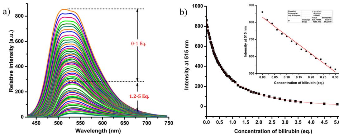
Fig. 7 (a) Emission spectra of 33  $\mu\text{M}$  solution of **9** in the presence of an increasing concentration of bilirubin in DMSO ( $\lambda_{\text{ex}} = 430 \text{ nm}$ ); (b) the plot of bilirubin concentration versus emission intensity at 538 nm (inset: The linear range).
