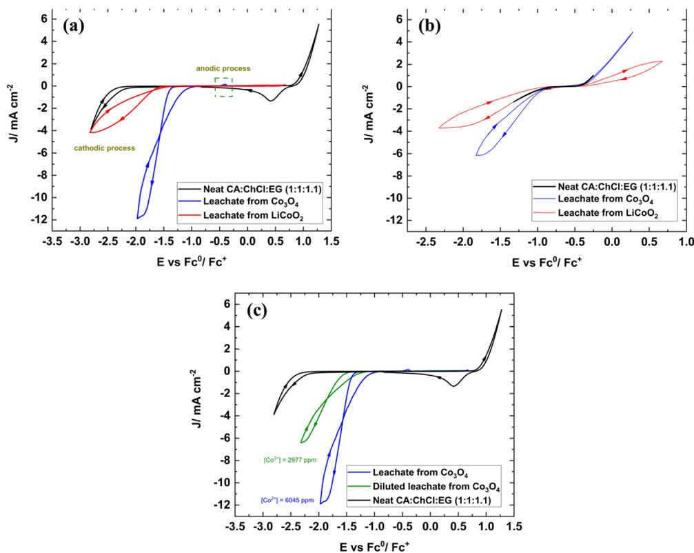
Fig. 4 Cyclic voltammograms corresponding to cobalt(II) in the leachates from  $\text{Co}_3\text{O}_4$  and  $\text{LiCoO}_2$  and the neat CA:ChCl:EG (1:1:1.1) using (a) GC working electrode and (b) Ni working electrode and (c) comparison of the  $\text{Co}_3\text{O}_4$  leachate with diluted  $\text{Co}_3\text{O}_4$  leachate using the GC working electrode. Scan rate:  $50\text{ mV s}^{-1}$  and temperature:  $60^\circ\text{C}$ .
