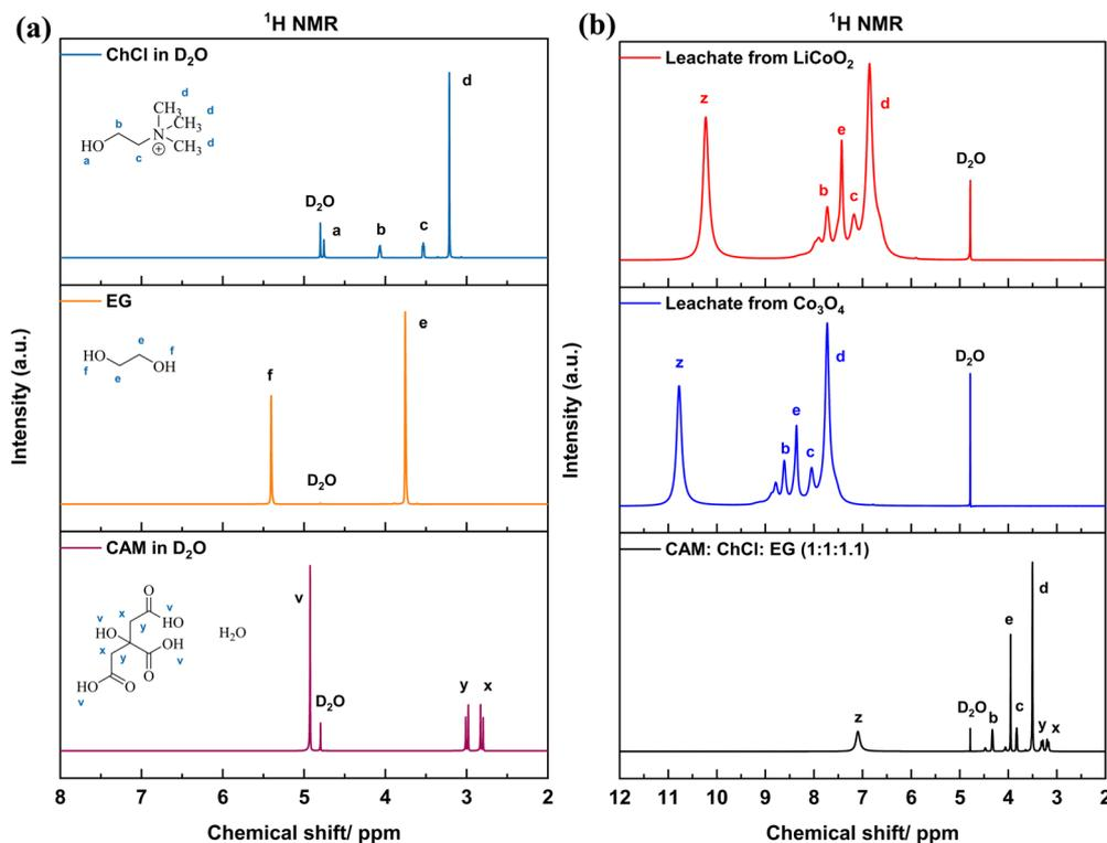
Fig. 5 (a) <sup>1</sup>H NMR spectra of ChCl dissolved in D<sub>2</sub>O (top), EG (middle), and CA dissolved in D<sub>2</sub>O (bottom) at 60 °C. (b) <sup>1</sup>H NMR spectra of CA:ChCl:EG (1:1:1.1) (bottom), leachate from Co<sub>3</sub>O<sub>4</sub> (middle) and the leachate from LiCoO<sub>2</sub> (top) analysed at 60 °C.
