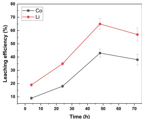
Fig. 3 Cobalt and lithium leaching efficiencies from  $\text{LiCoO}_2$  using CA:ChCl:EG (1:1:1.1) at S:L ratio = 1:66, 700 rpm,  $60^\circ\text{C}$  and different times.
