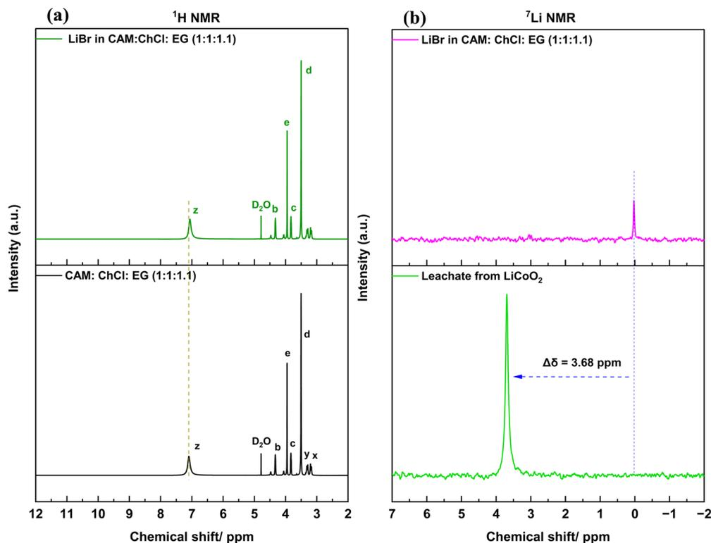
Fig. 6 (a)  $^1\text{H}$  NMR spectra of CA:ChCl:EG (1:1:1.1) and LiBr dissolved in CA:ChCl:EG (1:1:1.1) analysed at 60 °C and (b)  $^7\text{Li}$  NMR spectra of LiBr dissolved in CA:ChCl:EG (1:1:1.1) and the leachate from  $\text{LiCoO}_2$  analysed at 60 °C.
