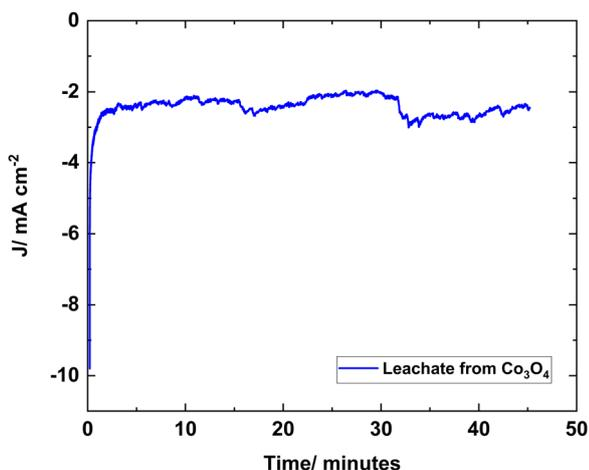
Fig. 7 Chronoamperometric response corresponding to the leachate from  $\text{Co}_3\text{O}_4$  on an Ni foil. Deposition time: 45 minutes at 60 °C.
