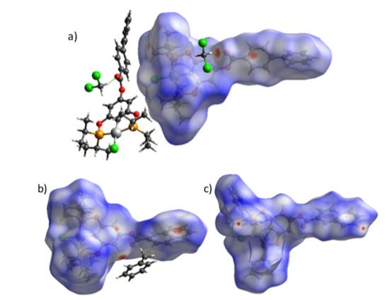
Fig. 4 Hirshfeld surface mapped over  $d_{\text{norm}}$  for compounds (a) 4 (b) 8 and (c) 9.
