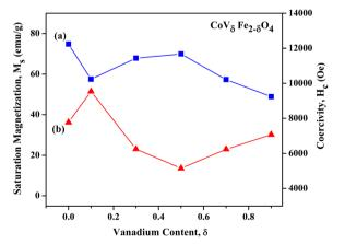
Fig. 15 Plots of the variation in (a)  $M_s$  and (b)  $H_c$  measured at 5 K for various V contents,  $\delta$  = 0.0, 0.1, 0.3, 0.5, 0.7 and 0.9 in  $CoV_{\delta}Fe_{2-\delta}O_4$ nanomaterials
