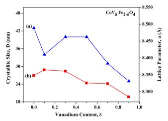
Fig. 3 Variation in (a) crystallite sizes, D, and (b) lattice parameters, a, with increasing V content ' $\delta$ ' in CoV $_{\delta}$ Fe $_{2-\delta}$ O $_{4}$  (0.0  $\leq \delta \leq$  0.9) nanomaterials annealed at 700 °C in an air atmosphere
