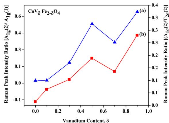
Fig. 9 Plots of Raman peak intensity ratios vs. vanadium content,  $\delta$ , in  $\text{CoV}_\delta\text{Fe}_{2-\delta}\text{O}_4$  ( $0.0 \leq \delta \leq 0.9$ ) nanomaterials: (a)  $A_{1g}(2)/A_{1g}(1)$  and (b)  $A_{1g}(2)/T_{2g}(2)$ .
