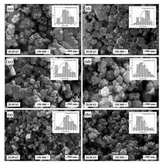
Fig. 10 FESEM micrographs for  $CoV_{\delta}Fe_{2-\delta}O_4$  nanomaterials annealed at 700 °C for different vanadium contents,  $\delta$ : (a) 0.0, (b) 0.1, (c) 0.3, (d) 0.5, (e) 0.7 and (f) 0.9 (insets present histograms of particle-size distributions in the respective  $CoV_{\delta}Fe_{2-\delta}O_4$  nanomaterials).
