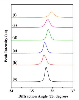
Fig. 2 Shift in the (311) line for  ${\rm CoV}_{\delta}{\rm Fe}_{2-\delta}{\rm O}_4$  (0.0  $\leq \delta \leq$  0.9) nanomaterials annealed at 700 °C for different vanadium contents,  $\delta$ : (a) 0.0, (b) 0.1, (c) 0.3, (d) 0.5, (e) 0.7 and (f) 0.9
