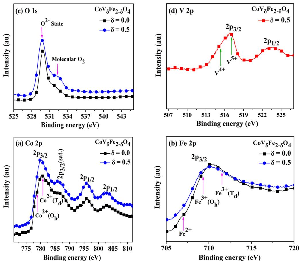
Fig. 11 XPS spectra of  $\text{CoV}_\delta\text{Fe}_{2-\delta}\text{O}_4$  nanomaterials (annealed at  $700^\circ\text{C}$ ) for (a) Co-2p, (b) Fe-2p, (c) O-1s for  $\delta = 0$  and (d) V-2p for  $\delta = 0.5$ .
