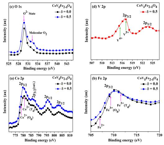
Fig. 11 XPS spectra of  $CoV_{\delta}Fe_{2-\delta}O_4$  nanomaterials (annealed at 700 °C) for (a) Co-2p, (b) Fe-2p, (c) O-1s for  $\delta=0$  and (d) V-2p for  $\delta=0.5$ .
