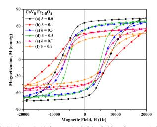
Fig. 14 M vs. H plots (measured at 5 K) for  $CoV_{\delta}Fe_{2-\delta}O_4$  nanomaterials annealed at 700 °C for different contents of vanadium,  $\delta$ : (a) 0.0, (b) 0.1, (c) 0.3, (d) 0.5, (e) 0.7 and (f) 0.9
