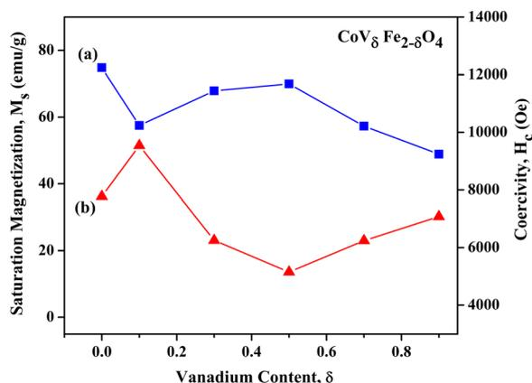
**Fig. 15** Plots of the variation in (a)  $M_s$  and (b)  $H_c$  measured at 5 K for various V contents,  $\delta = 0.0, 0.1, 0.3, 0.5, 0.7$  and  $0.9$  in  $\text{CoV}_\delta\text{Fe}_{2-\delta}\text{O}_4$  nanomaterials.
