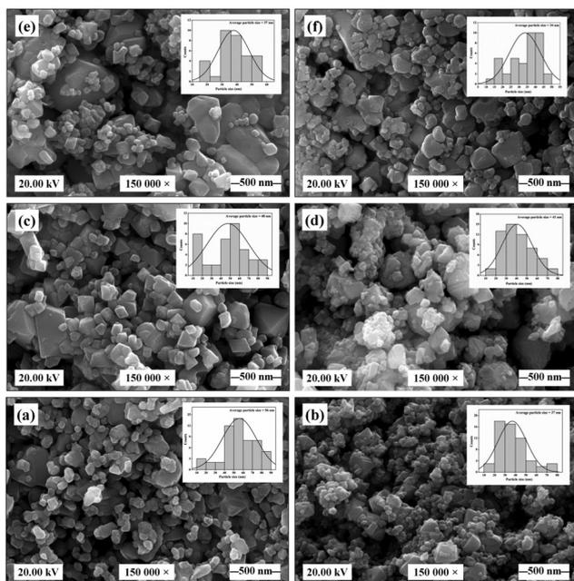
Fig. 10 FESEM micrographs for  $\text{CoV}_\delta\text{Fe}_{2-\delta}\text{O}_4$  nanomaterials annealed at  $700^\circ\text{C}$  for different vanadium contents,  $\delta$ : (a) 0.0, (b) 0.1, (c) 0.3, (d) 0.5, (e) 0.7 and (f) 0.9 (insets present histograms of particle-size distributions in the respective  $\text{CoV}_\delta\text{Fe}_{2-\delta}\text{O}_4$  nanomaterials).
