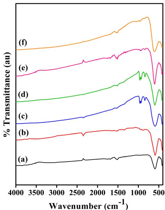
Fig. 6 FTIR spectra of  $\text{CoV}_\delta\text{Fe}_{2-\delta}\text{O}_4$  nanomaterials annealed at  $700\text{ }^\circ\text{C}$  for different vanadium contents,  $\delta$ : (a) 0.0, (b) 0.1, (c) 0.3, (d) 0.5, (e) 0.7 and (f) 0.9.
