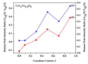
Fig. 9 Plots of Raman peak intensity ratios vs. vanadium content,  $\delta$ , in  $CoV_{\delta}Fe_{2-\delta}O_4$  (0.0  $\leq \delta \leq$  0.9) nanomaterials: (a)  $A_{1q}(2)/A_{1q}(1)$  and (b)  $A_{1q}(2)/A_{1q}(1)$  $T_{2g}(2)$
