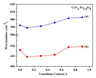
Fig. 7 Variation of IR frequencies as a function of vanadium content ( $\delta$ ) in  $CoV_{\delta}Fe_{2-\delta}O_4$  (0.0  $\leq \delta \leq$  0.9) nanomaterials annealed at 700 °C for various coordination sites: (a) tetrahedral site and (b) octahedral site
