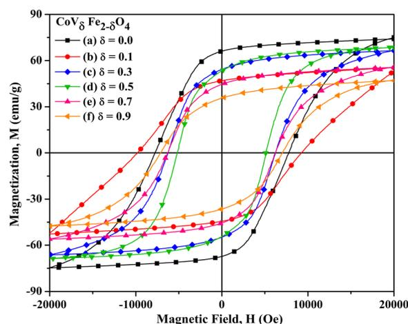
Fig. 14  $M$  vs.  $H$  plots (measured at 5 K) for  $CoV_\delta Fe_{2-\delta}O_4$  nanomaterials annealed at  $700 \text{ }^\circ\text{C}$  for different contents of vanadium,  $\delta$ : (a) 0.0, (b) 0.1, (c) 0.3, (d) 0.5, (e) 0.7 and (f) 0.9.
