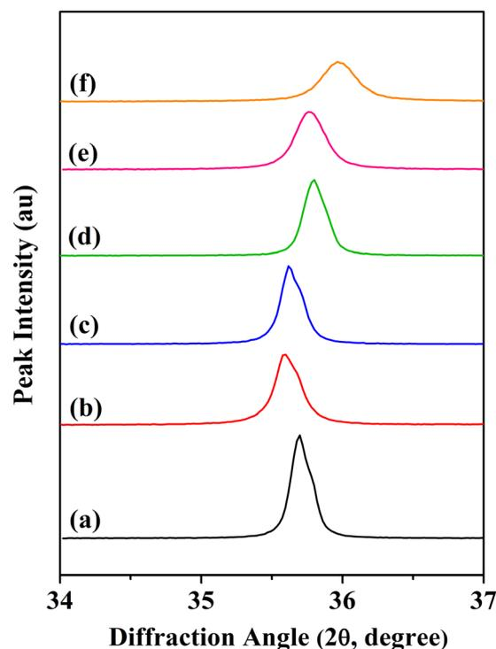
Fig. 2 Shift in the (311) line for  $\text{CoV}_\delta\text{Fe}_{2-\delta}\text{O}_4$  ( $0.0 \leq \delta \leq 0.9$ ) nanomaterials annealed at 700 °C for different vanadium contents,  $\delta$ : (a) 0.0, (b) 0.1, (c) 0.3, (d) 0.5, (e) 0.7 and (f) 0.9.
