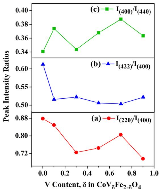
Fig. 5 XRD peak intensity ratios vs. vanadium content,  $\delta$ , in  $\text{CoV}_\delta\text{Fe}_{2-\delta}\text{O}_4$  ( $0.0 \leq \delta \leq 0.9$ ) nanomaterials: (a)  $I_{(220)}/I_{(400)}$ , (b)  $I_{(422)}/I_{(400)}$  and (c)  $I_{(400)}/I_{(440)}$ .
