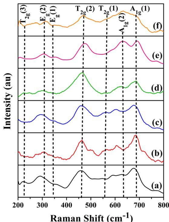
Fig. 8 Raman spectra for  $\text{CoV}_\delta\text{Fe}_{2-\delta}\text{O}_4$  nanomaterials annealed at  $700\text{ }^\circ\text{C}$  for different vanadium contents,  $\delta$ : (a) 0.0, (b) 0.1, (c) 0.3, (d) 0.5, (e) 0.7 and (f) 0.9.
