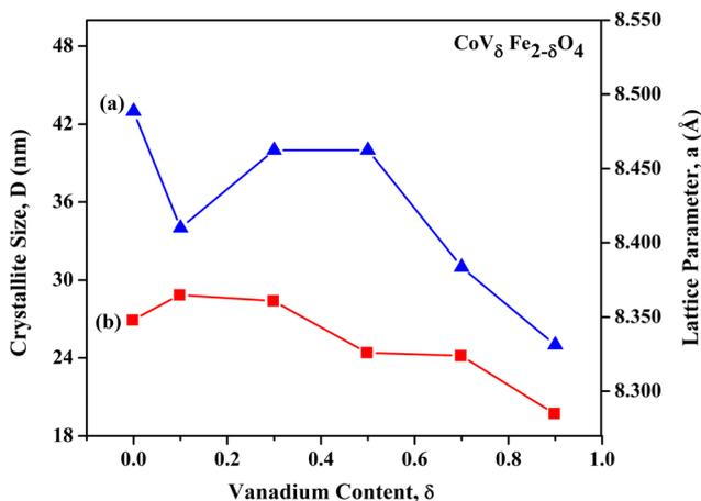
**Fig. 3** Variation in (a) crystallite sizes,  $D$ , and (b) lattice parameters,  $a$ , with increasing V content ' $\delta$ ' in  $\text{CoV}_\delta\text{Fe}_{2-\delta}\text{O}_4$  ( $0.0 \leq \delta \leq 0.9$ ) nanomaterials annealed at 700 °C in an air atmosphere.
