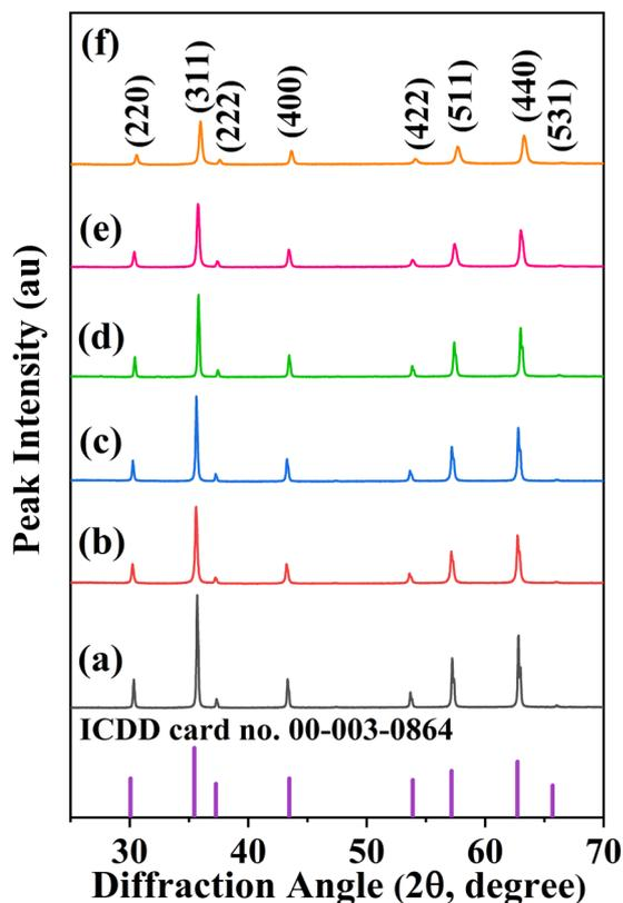
Fig. 1 XRD patterns of  $\text{CoV}_\delta\text{Fe}_{2-\delta}\text{O}_4$  ( $0.0 \leq \delta \leq 0.9$ ) nanomaterials annealed at 700 °C (air atmosphere) for different vanadium contents,  $\delta$ : (a) 0.0, (b) 0.1, (c) 0.3, (d) 0.5, (e) 0.7 and (f) 0.9 together with the XRD pattern for ICDD card no. 00-003-0864.
