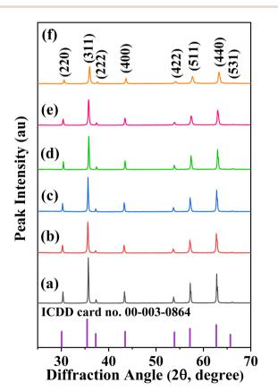
Fig. 1 XRD patterns of  $CoV_{\delta}Fe_{2-\delta}O_4$  (0.0  $\leq \delta \leq$  0.9) nanomaterials annealed at 700 °C (air atmosphere) for different vanadium contents,  $\delta$ : (a) 0.0, (b) 0.1, (c) 0.3, (d) 0.5, (e) 0.7 and (f) 0.9 together with the XRD pattern for ICDD card no. 00-003-0864.
