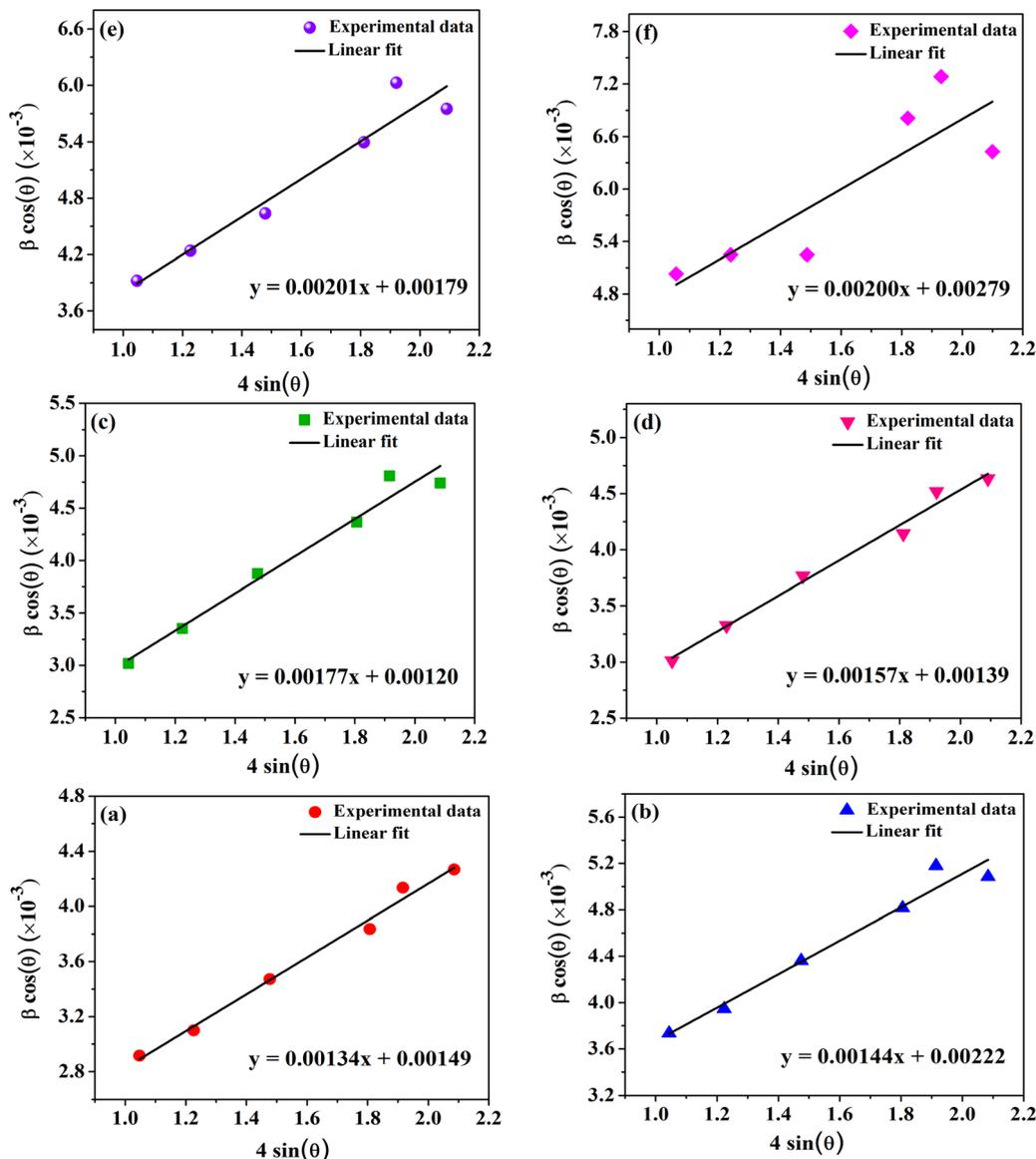
Fig. 4 Linearly fitted Williamson–Hall (WH) plots for  $\text{CoV}_\delta\text{Fe}_{2-\delta}\text{O}_4$  ( $0.0 \leq \delta \leq 0.9$ ) nanomaterials annealed at  $700^\circ\text{C}$  for different vanadium contents,  $\delta$ : (a) 0.0, (b) 0.1, (c) 0.3, (d) 0.5, (e) 0.7 and (f) 0.9.
