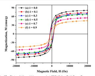
Fig. 12 Plots of M vs. H (measured at 300 K) for  $CoV_{\delta}Fe_{2-\delta}O_4$  nanomaterials annealed at 700 °C for different vanadium contents,  $\delta$ : (a) 0.0, (b) 0.1, (c) 0.3, (d) 0.5, (e) 0.7 and (f) 0.9.
