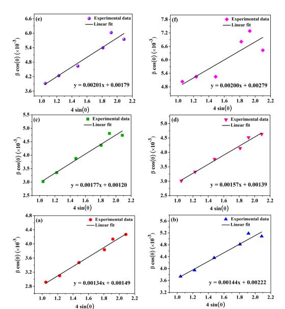
Fig. 4 Linearly fitted Williamson-Hall (WH) plots for CoV $_{\delta}$ Fe $_{2-\delta}$ O $_{4}$  (0.0  $\leq \delta \leq$  0.9) nanomaterials annealed at 700 °C for different vanadium contents,  $\delta$ : (a) 0.0, (b) 0.1, (c) 0.3, (d) 0.5, (e) 0.7 and (f) 0.9.
