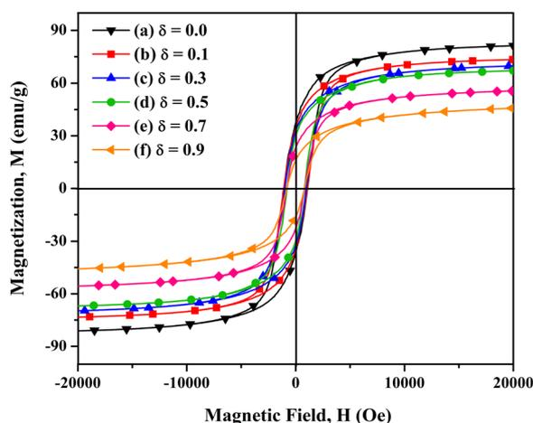
**Fig. 12** Plots of  $M$  vs.  $H$  (measured at 300 K) for  $\text{CoV}_\delta\text{Fe}_{2-\delta}\text{O}_4$  nanomaterials annealed at 700 °C for different vanadium contents,  $\delta$ : (a) 0.0, (b) 0.1, (c) 0.3, (d) 0.5, (e) 0.7 and (f) 0.9.
