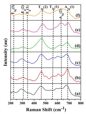
Fig. 8 Raman spectra for  $CoV_{\delta}Fe_{2-\delta}O_4$  nanomaterials annealed at 700 °C for different vanadium contents,  $\delta$ : (a) 0.0, (b) 0.1, (c) 0.3, (d) 0.5, (e) 0.7 and (f) 0.9.
