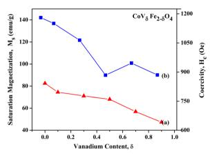
Fig. 13 Variation in magnetic parameters at room temperature (300 K) for  $CoV_{\delta}Fe_{2-\delta}O_4$  (0.0  $\leq \delta \leq$  0.9) nanomaterials: (a) saturation magnetization  $(M_s)$  and (b) coercivity  $(H_c)$ .
