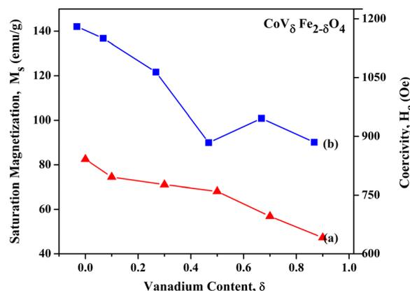
**Fig. 13** Variation in magnetic parameters at room temperature (300 K) for  $\text{CoV}_\delta\text{Fe}_{2-\delta}\text{O}_4$  ( $0.0 \leq \delta \leq 0.9$ ) nanomaterials: (a) saturation magnetization ( $M_s$ ) and (b) coercivity ( $H_c$ ).
