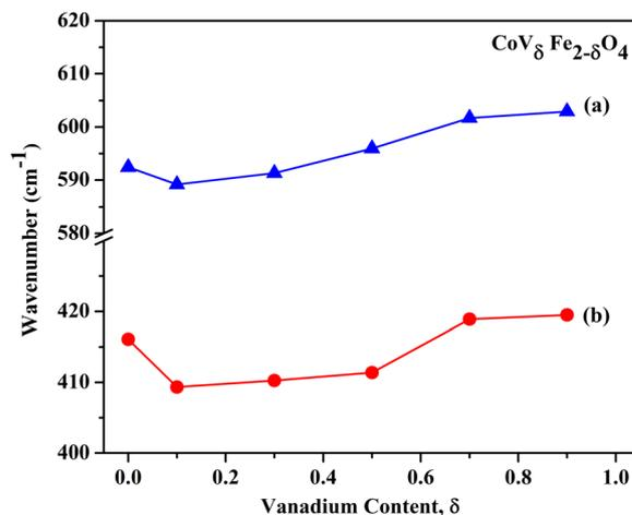
Fig. 7 Variation of IR frequencies as a function of vanadium content ( $\delta$ ) in  $\text{CoV}_\delta\text{Fe}_{2-\delta}\text{O}_4$  ( $0.0 \leq \delta \leq 0.9$ ) nanomaterials annealed at  $700\text{ }^\circ\text{C}$  for various coordination sites: (a) tetrahedral site and (b) octahedral site.
