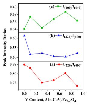
Fig. 5 XRD peak intensity ratios vs. vanadium content,  $\delta$ , in CoV $_{\delta}$ Fe $_{2-\delta}$ O $_{4}$  $(0.0 \le \delta \le 0.9)$  nanomaterials: (a)  $I_{(220)}/I_{(400)}$ , (b)  $I_{(422)}/I_{(400)}$  and (c)  $I_{(400)}/I_{(400)}$
