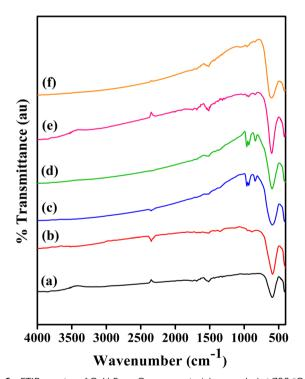
Fig. 6 FTIR spectra of  $CoV_{\delta}Fe_{2-\delta}O_4$  nanomaterials annealed at 700 °C for different vanadium contents,  $\delta$ : (a) 0.0, (b) 0.1, (c) 0.3, (d) 0.5, (e) 0.7 and (f) 0.9.
