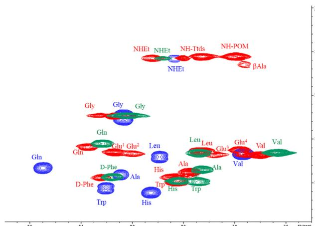
Fig. 4 Overlaid COSY spectra (in  $d_6$ -DMSO) for NH- $\text{CH}\alpha$  cross peaks belonging to free and  $V_6$ -grafted DB (Pep-1 (blue), POV-1 (green) and POV-4 (red)). The spectra were acquired on a Bruker DMX-600 instrument operating at 599.90 MHz for  $^1\text{H}$  at 298 K.
