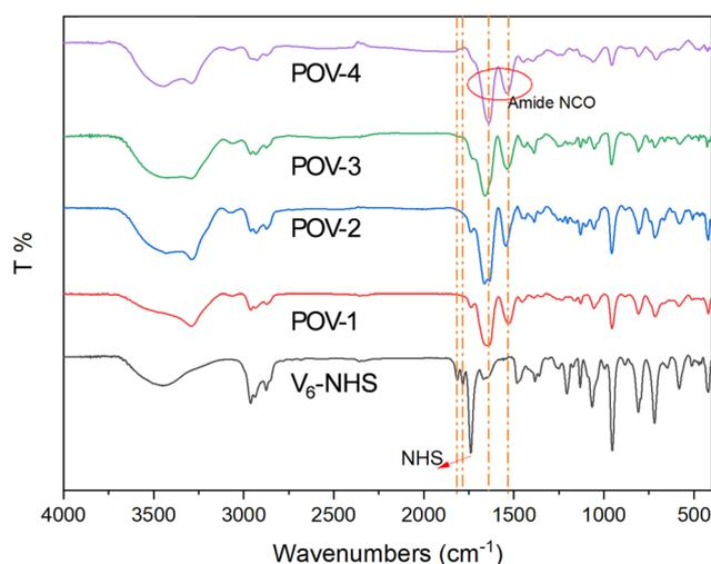
Fig. 2 FTIR (KBr) spectra of  $V_6$ -NHS (black), POV-1 (red), POV-2 (blue), POV-3 (green), POV-4 (purple), the orange dash-dot lines indicate the position of the characteristic peaks at  $1814\text{ cm}^{-1}$ ,  $1783\text{ cm}^{-1}$ ,  $1640\text{ cm}^{-1}$  and  $1534\text{ cm}^{-1}$  (see text).
