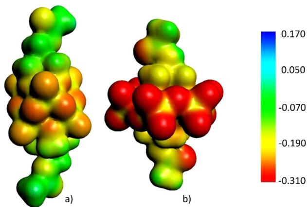
Fig. 1 DFT calculated electrostatic potential mapped on an electronic isosurface of 0.01 density for the two POM precursors: (a)  $[V_6O_{13}(OCH_2)_3CNH_2]^{2-}$  and (b)  $[MnMo_6O_{18}(OCH_2)_3CNH_2]^{3-}$ . Red and blue regions indicate negative and positive potential, respectively.
