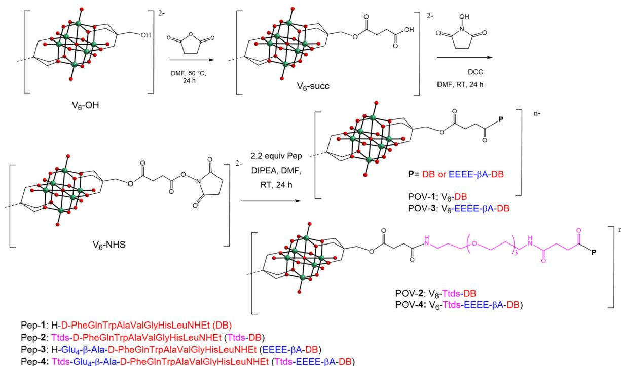
**Scheme 1** Reaction scheme to obtain the hybrid derivatives starting from  $\text{V}_6\text{-OH}$  ( $\text{TBA}_2[\text{V}_6\text{O}_{13}\{(\text{OCH}_2)_3\text{CH}_2\text{OH}\}_2]$ ). For clarity reasons, counter cations (TBA) are omitted.
