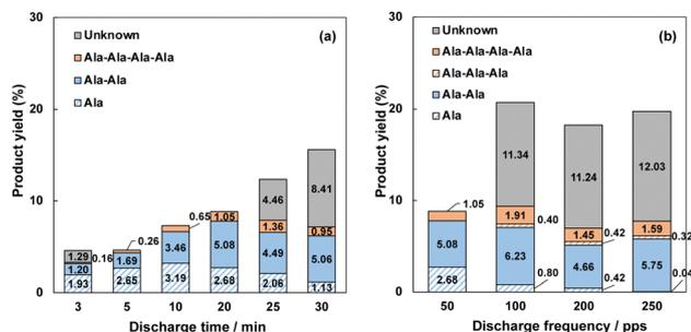
Fig. 1 Product yield from **Ala-DKP** at pH 4.6. (a) Influence of the discharge time and the (b) discharge frequency on the product yield. [**Ala-DKP**] = 100 mM (10 mL), initial pH: 4.6, discharge frequency: 50–250 pps, and discharge time: 3–30 min.
