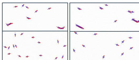
Snapshots of the particle configurations of surfactant-coated Co ferrite multicore (left), FeCo alloy (right) particles in the fluid by switching on (upper panels) an in-plane magnetic field at time  $t=10^8$  MCS and after switching off the field at  $t=1.1 \times 10^8$  MCS. Arrows show their corresponding spin orientation.
