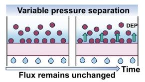
Piezoelectric PVDF membranes for emulsion separation with constant flux and high efficiency
