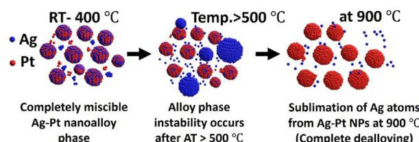
**Thermal evolution of solid solution of silica-embedded AgPt alloy NPs in the large miscibility gap**
