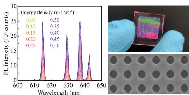
**High-refractive-index 2D photonic structures for robust low-threshold multiband lasing**
