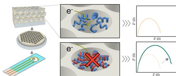
**Block copolymer-assembled nanopore arrays enable ultrasensitive label-free DNA detection**
