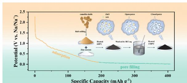
**Regulation of closed pores in hard carbon for enhanced electrochemical sodium storage**
