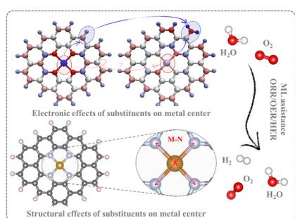
**Edge-doped substituents as an emerging atomic-level strategy for enhancing M–N<sub>4</sub>–C single-atom catalysts in electrocatalysis of the ORR, OER, and HER**
