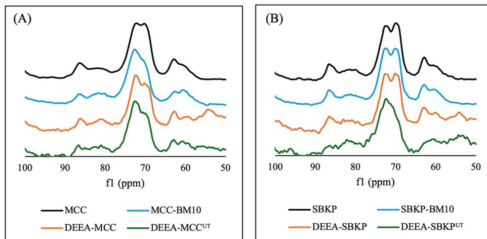
Fig. 2 SsNMR spectra of cellulose samples: starting materials, material milled neat for 10 min (BM10), aminoalkylated DEEA-substrates, and defibrillated DEEA-substrate<sup>UT</sup> (A) MCC, (B) SBKP.
