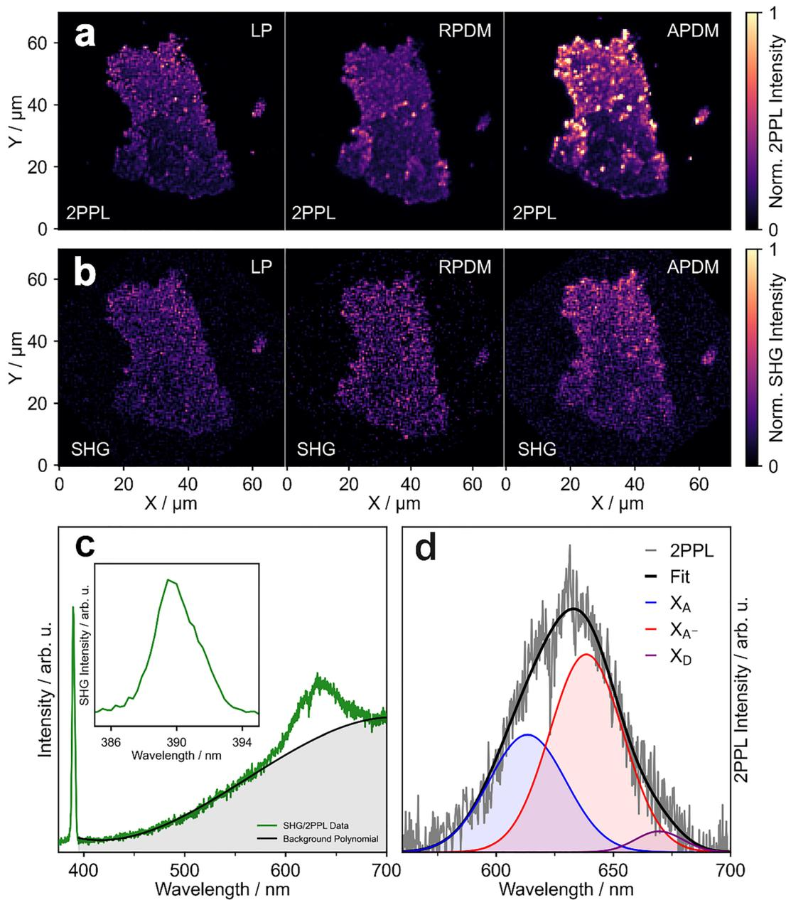
Fig. 3 (a) 2PPL intensity maps of WS<sub>2</sub> NS an agglomerate under LP, RPDM and APDM, resp. (b) SHG intensity maps of WS<sub>2</sub> NSs an agglomerate under LP, RPDM and APDM, resp. (c) 2PPL and SHG spectrum as collected by the nonlinear setup under APDM excitation. A background polynomial is fitted to allow subsequent fitting of the 2PPL contributions. (d) Fitted 2PPL spectrum (extracted from 3c) with three peaks associated to X, X<sub>A</sub><sup>-</sup>, and X<sub>D</sub>.
