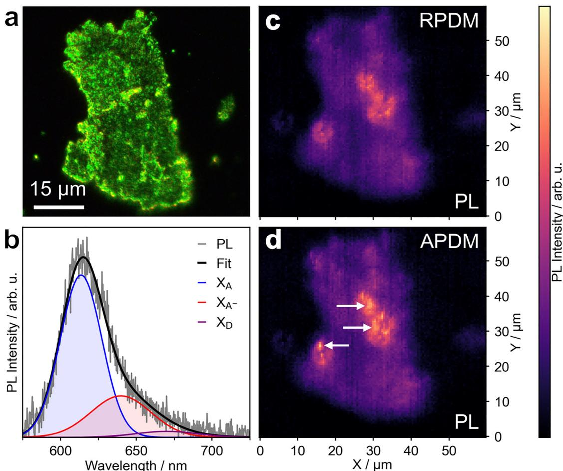
**Fig. 2** (a) Dark-field optical image of a  $WS_2$  NSs agglomerate. (b) PL spectrum of  $WS_2$  nanoflowers collected under APDM with fitted subpeaks, which can be attributed to  $X_A$ ,  $X_{A^-}$ , and  $X_D$ . (c) and (d) PL intensity maps of  $WS_2$  NS agglomerate shown in (a) under RPDM and APDM excitation, resp. White arrows highlight spots that are particularly bright under APDM excitation and indicate possibly flat-lying NSs with increased polarization-dependent PL intensity in APDM.
