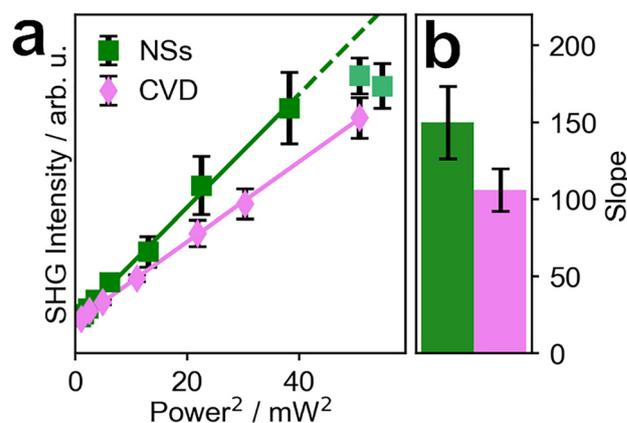
Fig. 4 (a) Power-dependent SHG intensity collected on deposited  $WS_2$  NSs. At high intensity, the  $WS_2$  NSs exhibit signs of photodamage (b) calculated slopes of  $WS_2$  NSs and CVD grown  $WS_2$  flakes shown in (a) with deposited  $WS_2$  NSs exhibiting a higher response on average.
