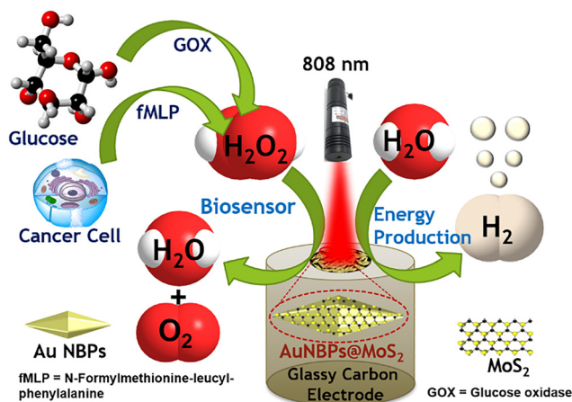
Scheme 1 Schematic representation of the enhanced electrochemical performances of AuNBPs@MoS 2 upon LSPR excitation.
