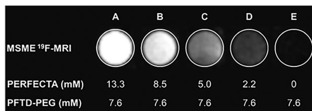
Fig. 2 Multi-slice multi-echo (MSME) sequence for  $^{19}\text{F}$ -MR imaging of PFTD-PEG micelles containing various concentrations of PERFECTA.
