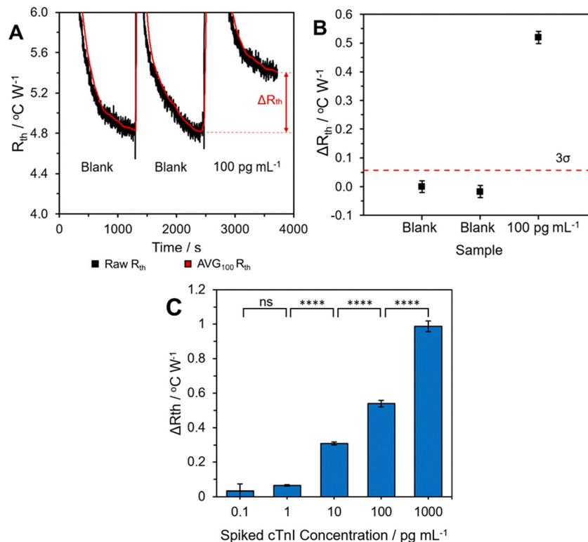
Fig. 4 (A) Typical raw (black) HTM data plot ( $R_{th}$  vs. time) with a moving average overlay (red), demonstrating the clear thermal response to the presence of cTnI. (B) Corresponding  $\Delta R_{th}$  plot. (C) Thermal detection of various cTnI concentrations (0.1–1000  $\text{pg mL}^{-1}$ ) in spiked human ISF samples.
