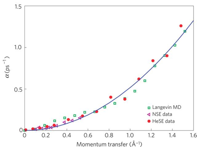
Fig. 9 Diffusion of 0.5 ML Benzene (C<sub>6</sub>H<sub>6</sub>) on graphite at 140 K follows Brownian motion. The dephasing rate  $\alpha$  obtained from HeSE measurements (circles), NSE measurements (triangles), and Langevin molecular dynamics (MD) simulations (squares) closely follows the parabolic fit (dark blue line), confirming the theoretical prediction of Brownian motion. (Reprinted with permission from ref. 68, Copyright 2009 by Springer Nature).
