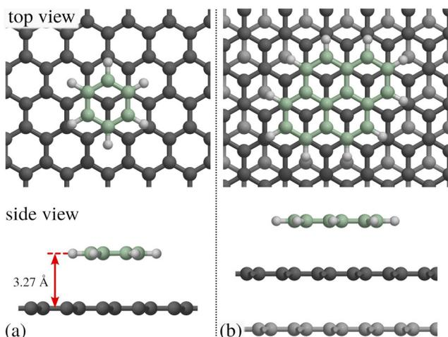
Fig. 7 (a) Top and side view of benzene ( $C_6H_6$ ) adsorbed on graphene, giving rise to the typical planar face-to-face adsorption geometry with an adsorption height of  $\approx 3.3 \text{ \AA}$ . (b) Similarly, pyrene ( $C_{16}H_{10}$ ) adsorbed on graphite adopts the AB stacking of the substrate. The carbon atoms of the aromatics are shown in light green for illustrative purposes.
