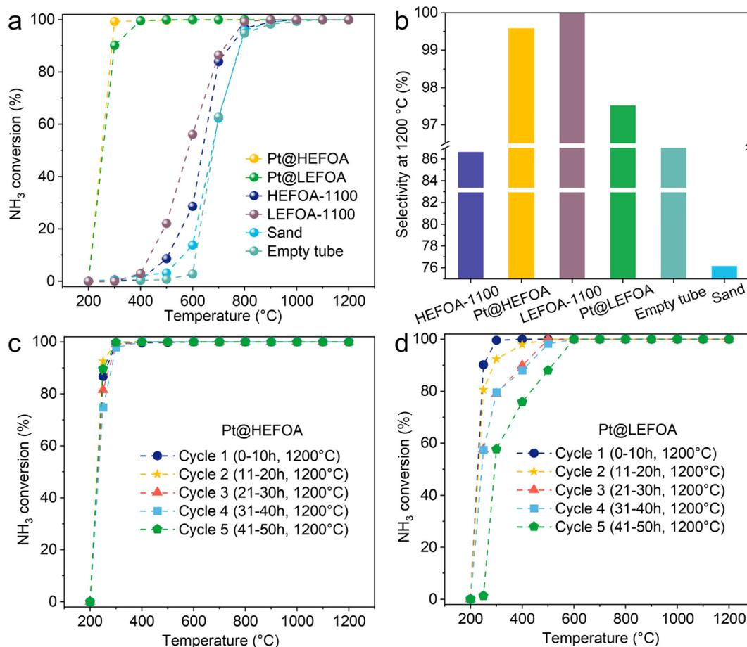
Fig. 6 HT-CAC performance of materials. (a)  $\text{NH}_3$  conversion at different temperatures. (b)  $\text{N}_2$  selectivity at 1200 °C. The  $\text{NH}_3$  conversion of (c) Pt@HEFOA and (d) Pt@LEFOA during 50-hours cycle stability tests. Reaction conditions for (a)–(d): 2 vol%  $\text{NH}_3$ , 3 vol%  $\text{O}_2$ , Ar balance, 100 mL  $\text{min}^{-1}$  flow rate,  $W/F = 2 \times 10^{-3}\text{ g min mL}^{-1}$ ,  $\text{GHSV} = 5500\text{ h}^{-1}$ .
