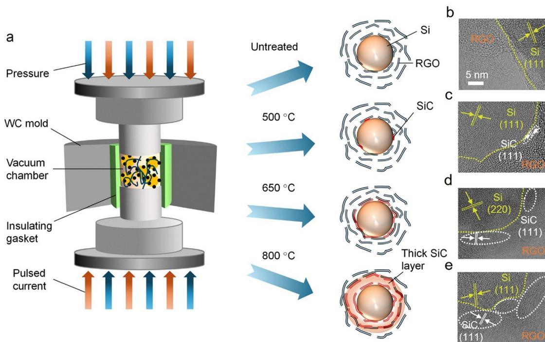
**Fig. 1** Schematic diagram of the preparation of Si-based composites by modified SPS technology. (a) Diagrammatic illustration of the modified SPS system and different RGO/Si composites prepared by adjusting the SPS temperature. (b)–(e) High-resolution TEM images of RGO/Si, S500, S650, and S800. Scale bars, 5 nm (b)–(e).
