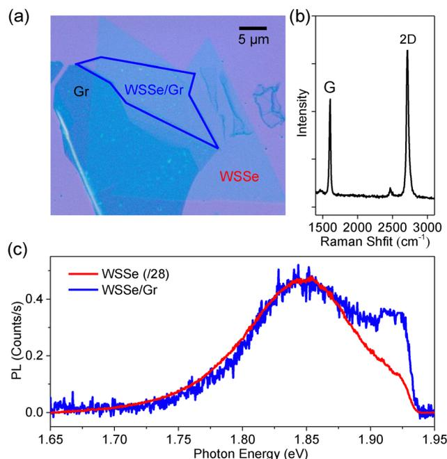
**Fig. 2** (a) Optical microscope image of the sample. The Janus WSSe/graphene heterostructure region is outlined in blue. (b) Raman spectrum of the graphene monolayer. (c) Photoluminescence (PL) spectra of the Janus WSSe monolayer and the heterostructure regions.
