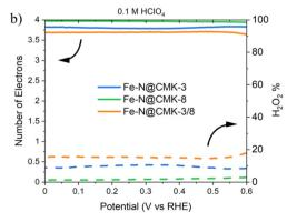
Fig. 6 ORR selectivity by RRDE measurement in (a) alkaline and (b) acidic environments.
