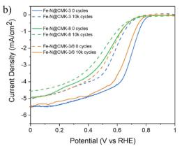
Fig. 7 LSV recorded before (0 cycles) and after (10k cycles) the durability test in both (a) alkaline and (b) acid electrolytes.
