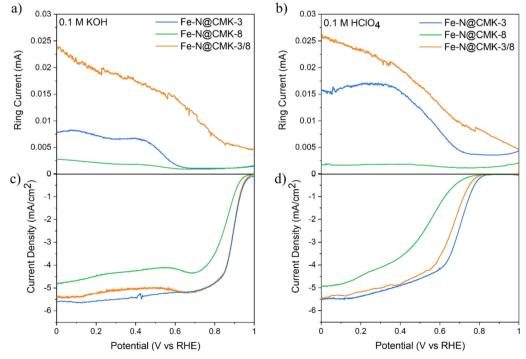
Fig. 5 ORR electrocatalytic activity recorded at 1600 rpm: (a) ring current in 0.1 M KOH. (b) Ring current in 0.1 M HClO<sub>4</sub>. (c) Disk current density in 0.1 M KOH. (d) Disk current density in 0.1 M HClO<sub>4</sub>.
