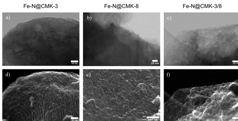
**Fig. 4** TEM images of (a) Fe–N@CMK-3, (b) Fe–N@CMK-8 and (c) Fe–N@CMK-3/8 electrocatalysts; and SEM images of the (d) Fe–N@CMK-3, (e) Fe–N@CMK-8 and (f) Fe–N@CMK-3/8 electrocatalysts.
