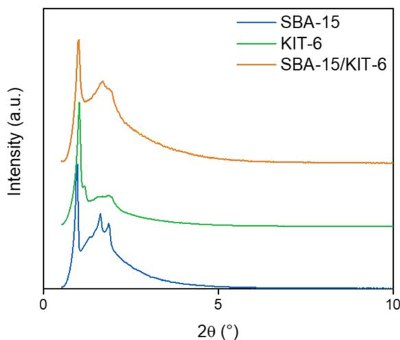
**Fig. 1** PXRD of the synthesized sacrificial silica templates.
