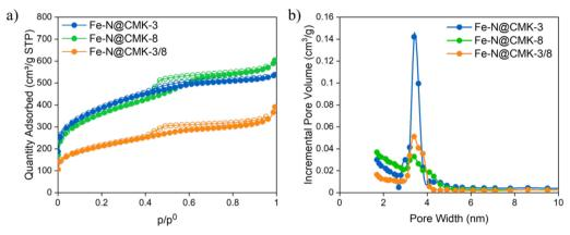
Fig. 3 (a) -196 °C N<sub>2</sub> adsorption-desorption isotherms of the Fe-N@C catalysts. Full symbols are related to the adsorption branches; empty symbols correspond to desorption ones. (b) Pore size distribution curves.
