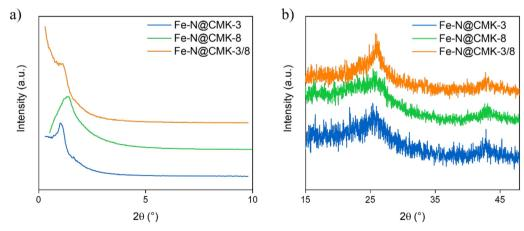
Fig. 2 (a) Low-angle PXRD of the Fe-N@C electrocatalysts acquired under transmission mode; (b) high-angle PXRD of the Fe-N@C electrocatalysts obtained under reflection mode.
