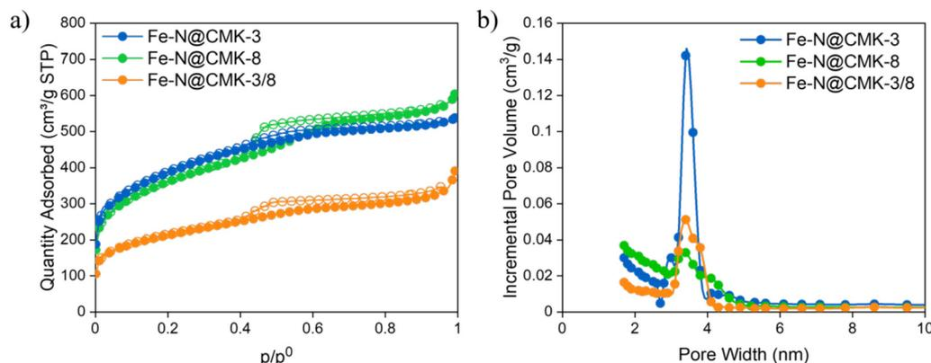
**Fig. 3** (a) –196 °C N<sub>2</sub> adsorption–desorption isotherms of the Fe–N@C catalysts. Full symbols are related to the adsorption branches; empty symbols correspond to desorption ones. (b) Pore size distribution curves.
