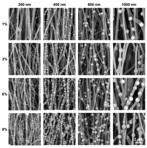
Fig. 1 SEM images of the different PCL/SiO<sub>2</sub> hybrid nanofibers. The SiO<sub>2</sub> protrusions on the fiber surfaces were defined as the "cell climbing stones".
