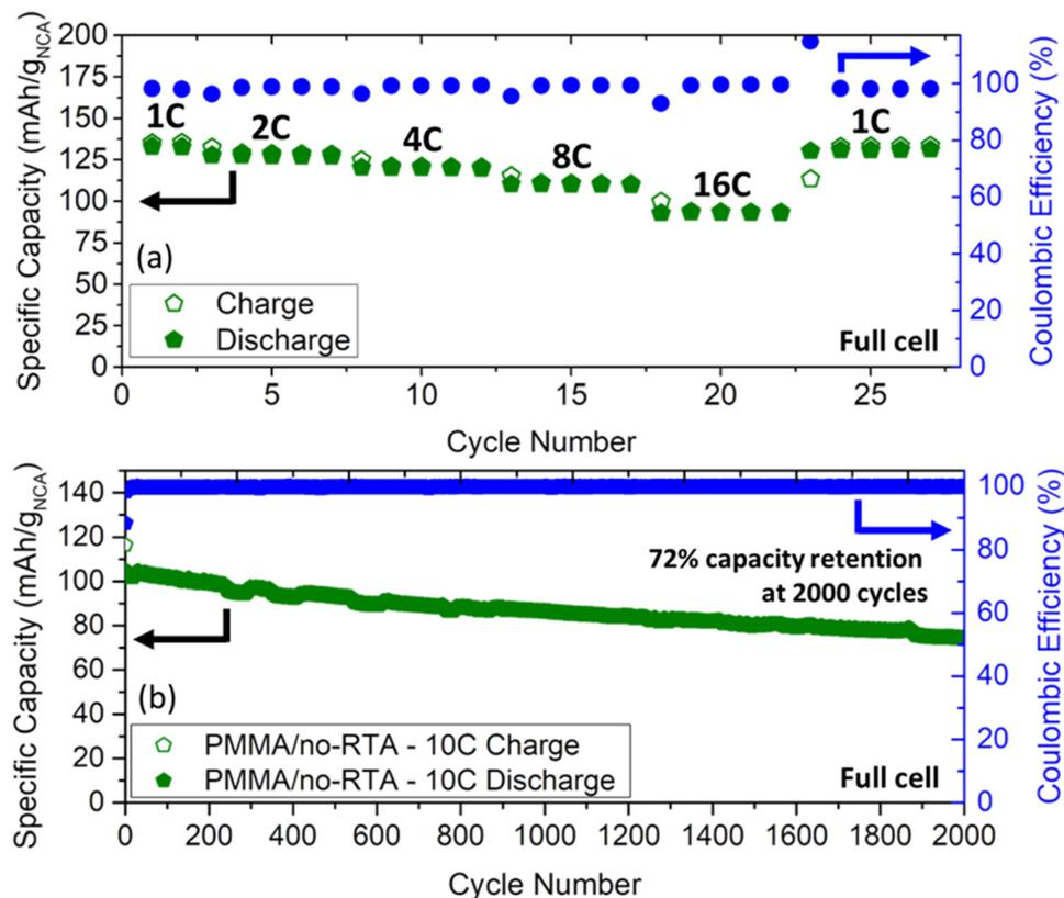
Fig. 5 Full-cell pseudocapacitor made with a PMMA/no-RTA NCA cathode and a Nb<sub>2</sub>O<sub>5</sub>-rGO anode cycled galvanostatically at various C-rates (a) and long-term cycling at 10C from 1.0–2.8 V (b). We observe 72% capacity retention after 2000 cycles. Specific capacity for charge is shown with open symbols, discharge with closed symbols, and the coulombic efficiency is shown in blue.
