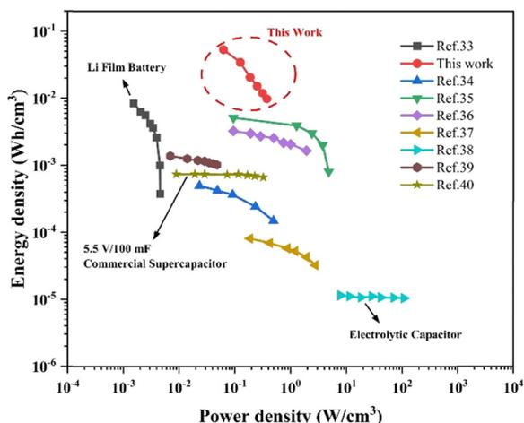
**Fig. 8** Ragone plots that compare the energy and power densities of micro/solid state flexible supercapacitors with those of commercial electrolytic capacitors, supercapacitors, and Li thin-film battery energy storage devices.<sup>33–40</sup>
