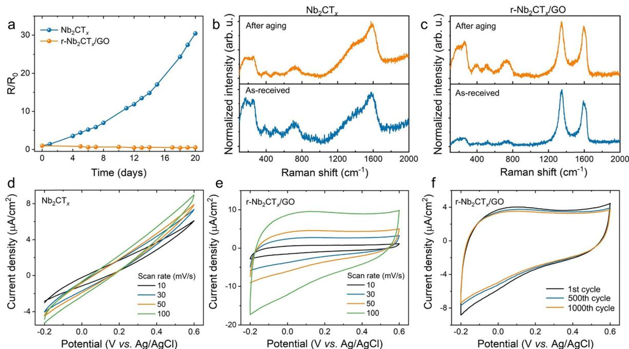
Fig. 4 (a) Evolution of the relative resistance of  $\text{Nb}_2\text{CT}_x$  and  $r\text{-Nb}_2\text{CT}_x/\text{GO}$  measured over time. Raman spectra of (b)  $\text{Nb}_2\text{CT}_x$  and (c)  $r\text{-Nb}_2\text{CT}_x/\text{GO}$  after aging. The CV curve of (d)  $\text{Nb}_2\text{CT}_x$  and (e)  $r\text{-Nb}_2\text{CT}_x/\text{GO}$  at different scan rates. (f) Cycling stability of  $r\text{-Nb}_2\text{CT}_x/\text{GO}$  at a scan rate of  $50 \text{ mV s}^{-1}$  up to 1000 CV cycles.
