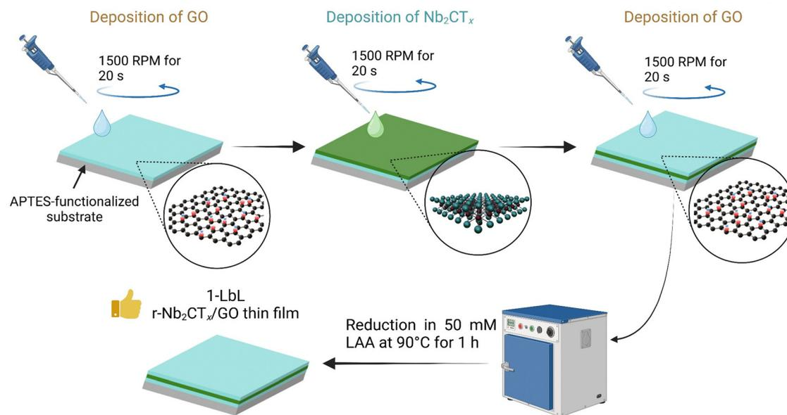
Fig. 1 Schematic of r-Nb<sub>2</sub>CT<sub>x</sub>/GO thin film fabrication. Partly created with BioRender.com.
