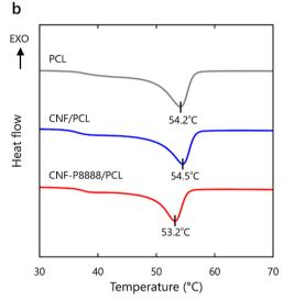
**Fig. 4** Crystallinity analyses. (a) XRD profiles and (b) DSC curves of pristine PCL, CNF-P8888/PCL, and CNF/PCL at 10% w/w CNF content.
