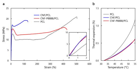
Fig. 3 Comparison of the reinforcing function between CNF-P8888 and pristine CNF. (a) Typical stress-strain curves and (b) thermal expansion curves of pristine PCL, CNF-P8888/PCL, and CNF/PCL at a 10% w/w CNF content.
