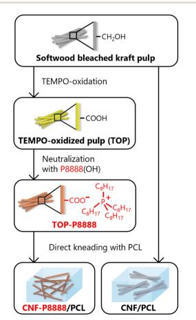
**Fig. 1** Schematic illustration for preparation procedure of the CNF-P8888/PCL and CNF/PCL composites.
