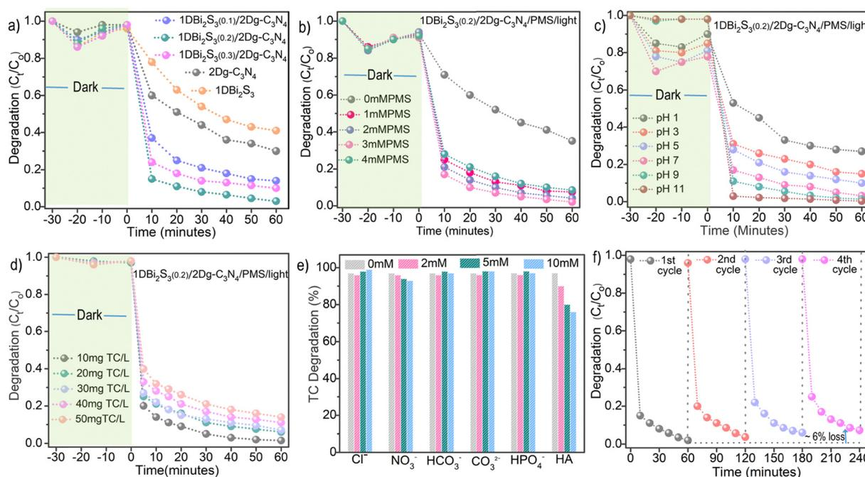
Fig. 5 Effect of various reaction parameters on the TC degradation: (a) 1D Bi<sub>2</sub>S<sub>3</sub> concentrations, (b) PMS concentration, (c) influence of pH, (d) TC concentration, (e) effect of common ions/molecules, and (f) recycling experiment.
