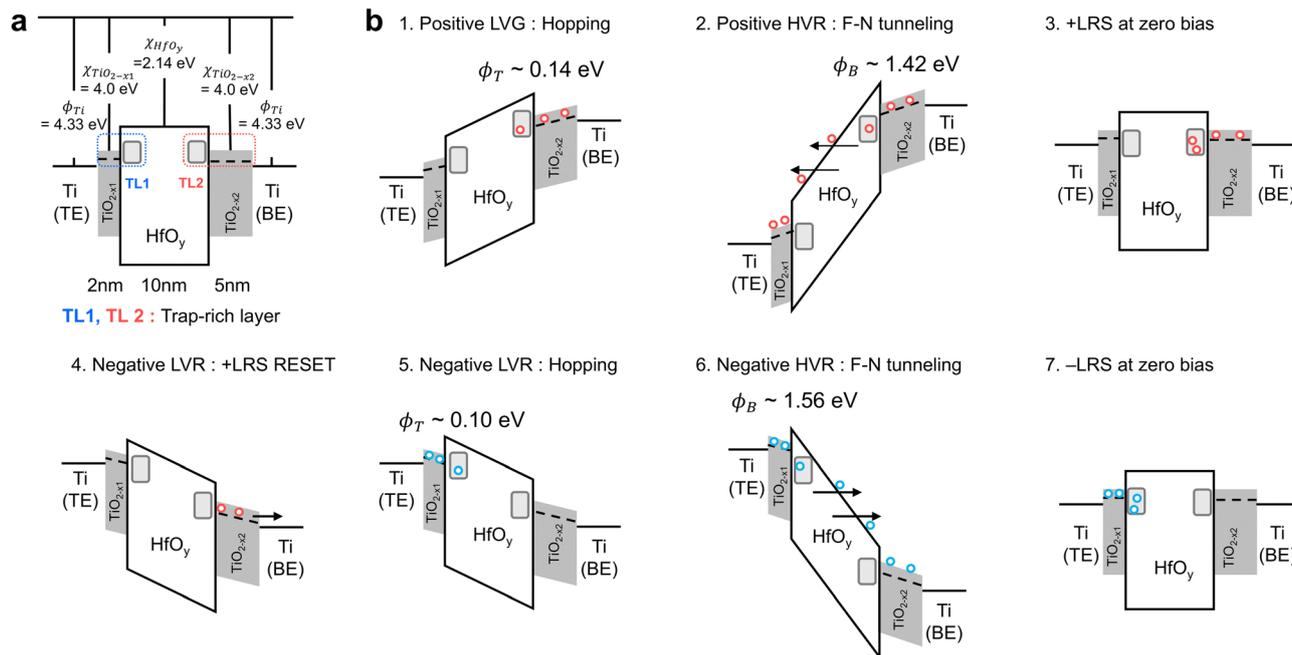
Fig. 5 (a) A schematic band diagram of the THT memristor under zero bias conditions. (b) Schematic band diagrams showing the +SET (steps 1 to 3), +RESET (step 4), and -SET (steps 5 to 7) mechanisms based on charge trapping/detrapping.
