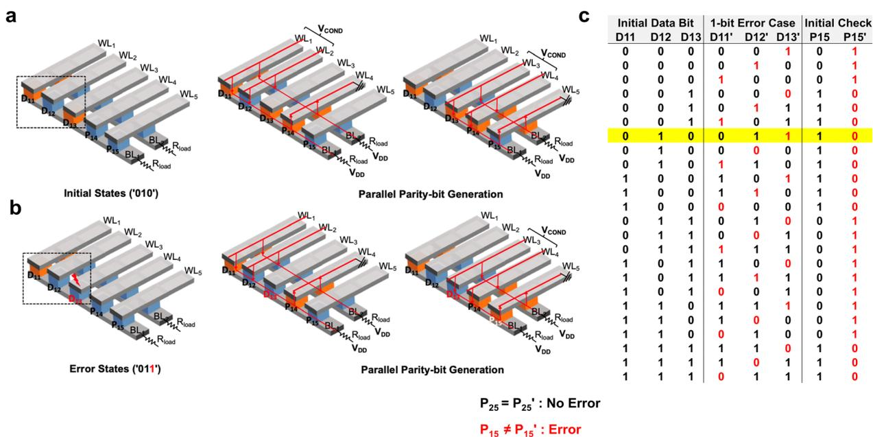
Fig. 9 Parallel error detection for three input data bits in  $2 \times 5$  memristors. The XNOR logic gates can be operated in parallel along the BL. (a) Parity-bit generation using two XNOR logic gates (b) The 1-bit error detection process when the  $BL_1$  data is flipped from '010' to '011'. (c) The parity bits for all possible 1-bit error cases for the three data bits.
