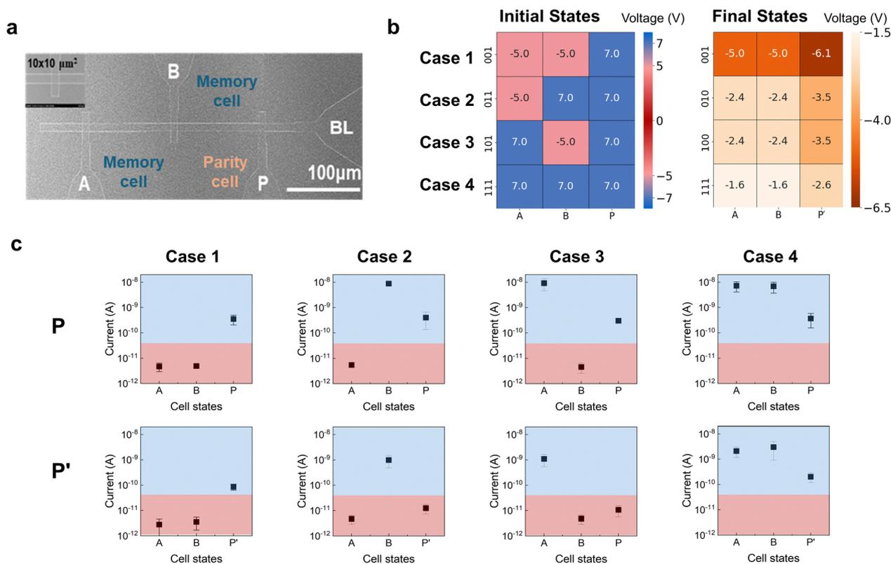
Fig. 8 Experimental demonstration of an XNOR logic gate. (a) A top-view SEM image of the  $1 \times 3$  THT memristor consisting of two input cells and an output cell. (b) The voltage drop across each memristor in the initial and final states for each XNOR logic gate input case. (c) The results from 15 cycles of the XNOR gate.
