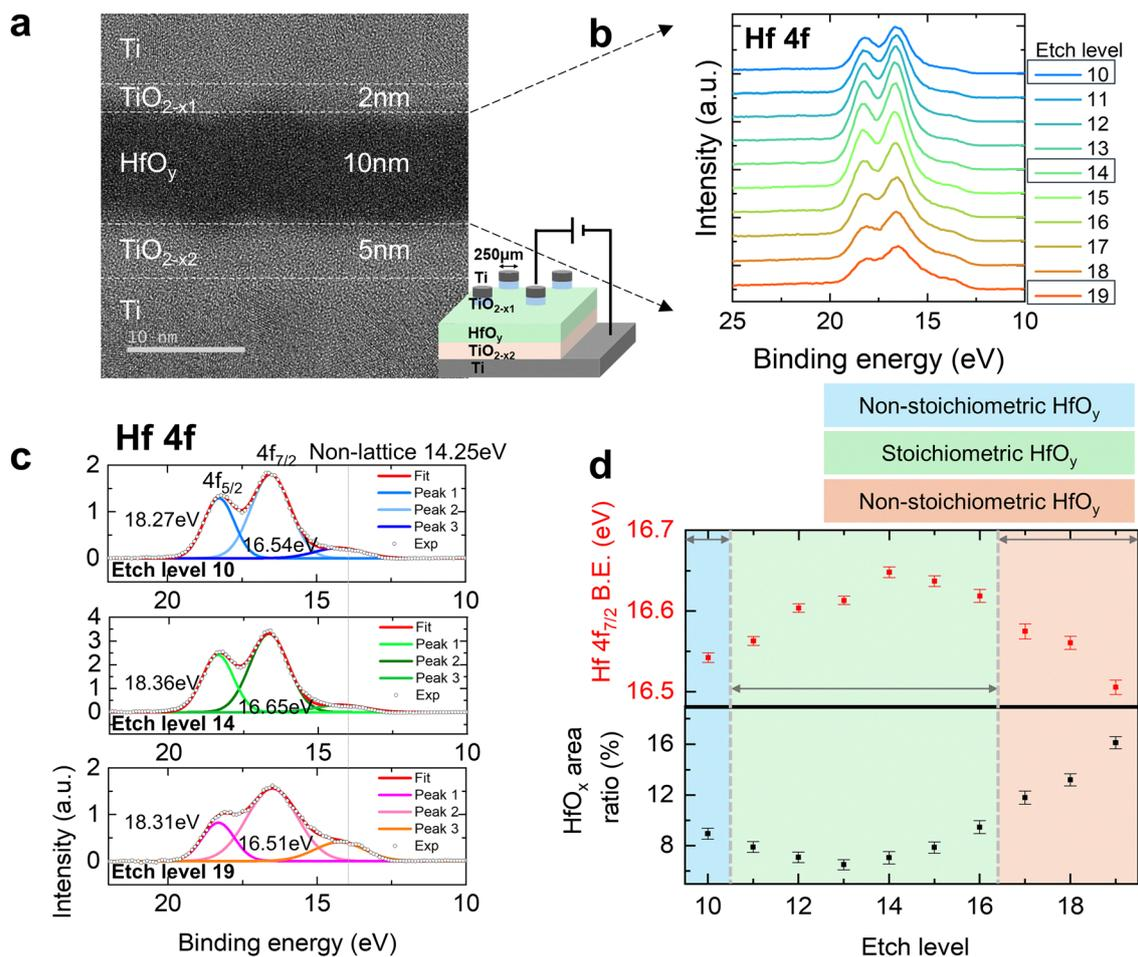
**Fig. 1** (a) A cross-sectional TEM image of the Ti/TiO<sub>2-x1</sub>/HfO<sub>y</sub>/TiO<sub>2-x2</sub>/Ti structure. (b) XPS spectra of the Hf 4f region for a depth profile of the HfO<sub>y</sub> layer. (c) Deconvolution of the Hf 4f peaks at etching levels of 10, 14, and 19. (d) Binding energy (upper panel) and HfO<sub>x</sub> area ratio (lower panel) shift analysis.
