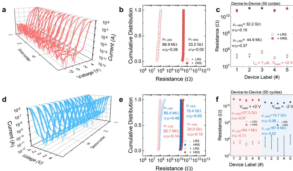
Fig. 3 (a) DC  $I$ - $V$  switching cycles of positive eBRS for 15 devices, each measured over 10 cycles. (b) Cycle-to-cycle variation of positive eBRS over 50 cycles. (c) Device-to-device variation of positive eBRS for 5 devices over 50 cycles. (d) DC  $I$ - $V$  switching cycles of eCRS for 15 devices, each measured over 10 cycles. (e) Cycle-to-cycle variation of eCRS over 50 cycles. (f) Device-to-device variation of eCRS for 5 devices over 50 cycles.
