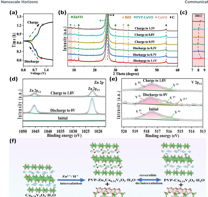
Fig. 6 (a) Discharge/charge curves of PVP-CaVO in AZIBs. (b) Ex situ XRD patterns. (c) Enlargements of patterns. (d) XPS spectra of Zn 2p. (e) XPS spectra of V 2p. (f) Schematic illustration of the Zn<sup>2+</sup> storage mechanism of PVP-CaVO
