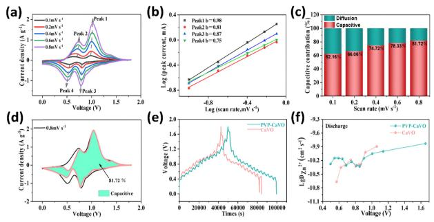
Fig. 5 (a) CV profiles of PVP-CaVO. (b) Correlation between log(i) and log(v) corresponding to the redox peaks of the PVP-CaVO electrode. (c) Capacitance contribution at different scan rates. (d) Capacitive contribution at 0.8 mV s<sup>-1</sup> of PVP-CaVO. (e) GITT curves of CaVO and PVP-CaVO. (f) Zn<sup>2+</sup> diffusion coefficient ( $D_{Zn^{2+}}$ ) of CaVO and PVP-CaVO.
