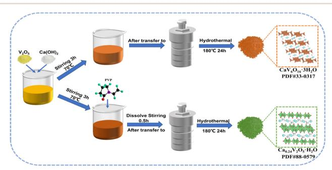
Fig. 1 Preparation process of CaVO and PVP-CaVO.
