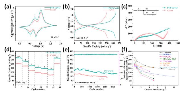
Fig. 4 (a) CV curves of CaVO and PVP-CaVO at 0.8 mV s<sup>-1</sup>. (b) GCD curves of CaVO and PVP-CaVO at 0.5 A g<sup>-1</sup>. (c) Comparison of the Nyquist plots of CaVO and PVP-CaVO before cycling. (d) Rate performance comparison of CaVO and PVP-CaVO. (e) Cycling performance comparison of CaVO and PVP-CaVO. (f) Comparison of the discharge specific capacity of PVP-CaVO as a cathode with other reported cathodes used in aqueous zinc-ion batteries
